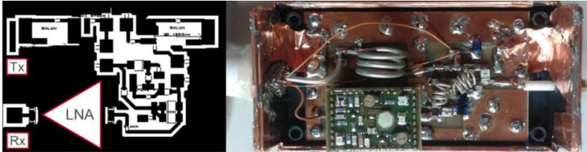
**Fig. A.11:** PCB layout of 70x90 mm<sup>2</sup> (left) and photo of the prototype of the linear Tx/Rx switch (right).
