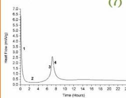
A narrow peak was observed between 6 and 8 hrs by isothermal calorimetry (at 25 °C, Fig. 7), which we attribute to a low sulfate content. Future formulations will include 1 wt% gypsum [Ca(SO<sub>4</sub>)<sub>2</sub>] to extend the kinetics of the hydration reaction.
