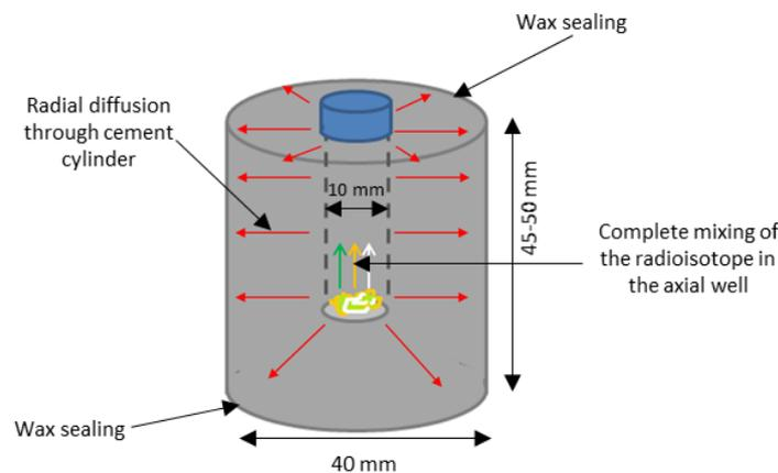
Figure 1: Schematic of the radial diffusion experiments.
