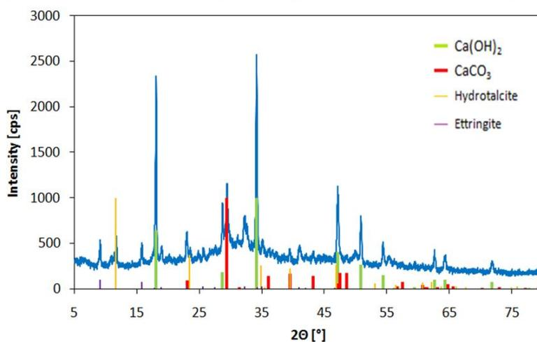
**Figure 2:** XRD spectrum of the hydrated cement A.
