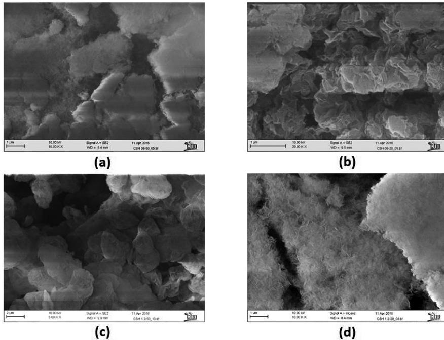
**Figure 3:** SEM images obtained for C-S-H gels: **(a)** Sample C/S 0.8 - S/L 50 at 10 kx; **(b)** Sample C/S 0.8 – S/L 20 at 20 kx; **(c)** Sample C/S 1.2 – S/L 50 at 5 kx; **(d)** Sample C/S 1.2 - S/L=20 at 10 kx.
