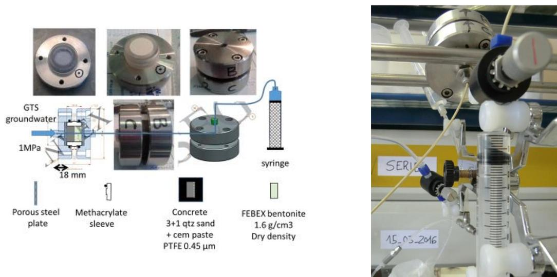
**Figure 4:** Scheme and details of the SERIE experiments.
