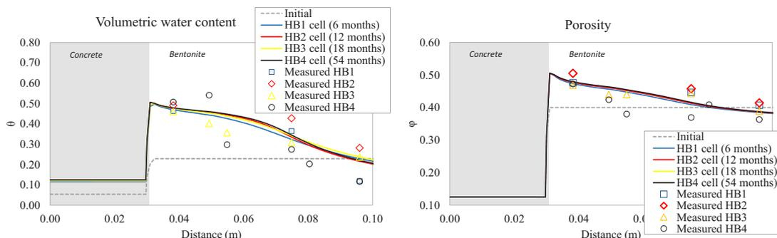
**Figure 2:** Computed (lines) volumetric water content (left) and porosity (right) and measured data (symbols) for the HB1, HB2, HB3, and HB4 cells.
