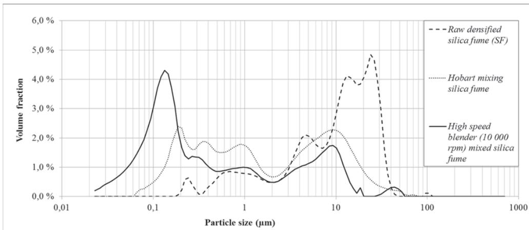
**Figure 5:** Dispersion state of SF in its densified state, after planetary mixing, and after high-speed mixing.
