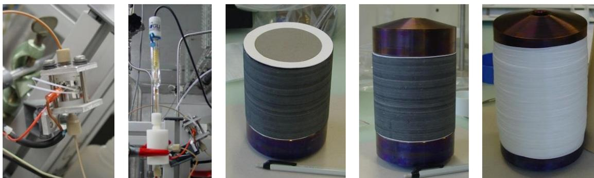
**Figure 2:** *From left:* electric conductivity cell; pH cell; sample with Ti filter (grey) and PTFE annulus; core assembly with sample (Opalinus Clay) between filters and Ti adapters; sample assembly wrapped in Teflon tape.
