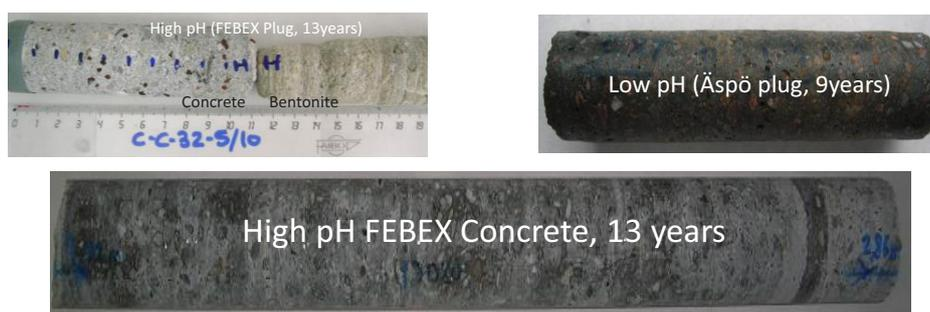
**Figure 1:** Concrete samples for aging characterisation of degradation. **Up-left)** FEBEX concrete 13y age bentonite-waters interaction, **Up-right)** Low pH Concrete from Äspö site (9 y age), **Down)** FEBEX concrete plug 13 y age.
