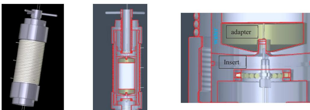
**Figure 1:** Core infiltration apparatus with thermostat coil (**left**), cross section (**middle**) and details (**right**): sample (white), titanium adapter (grey-green metallic), steel insert (label) and fittings to feed a capillary to the filter disc located between sample and adapter.
