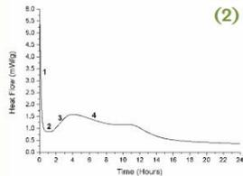
Isothermal calorimetry was performed at 25 °C within minutes of mixing the paste (Fig. 2). Several thermal features were identified:
