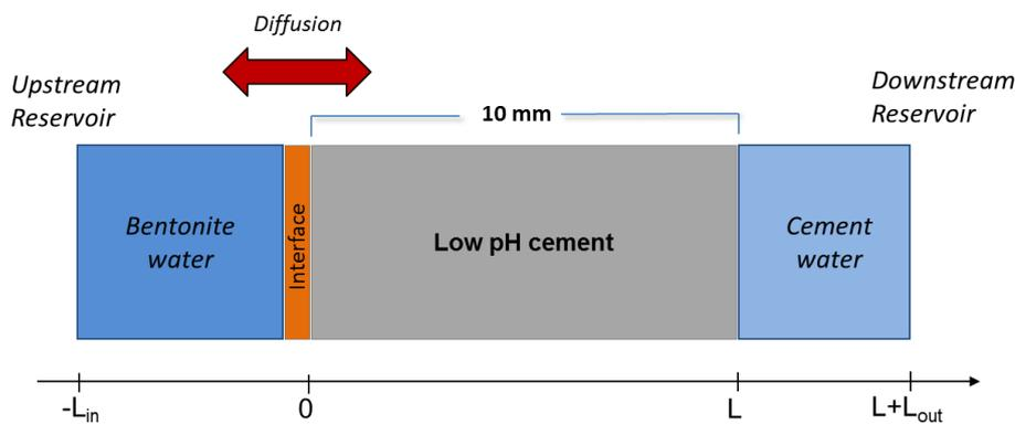
Figure 1: Schematic representation of the diffusion experiments.
