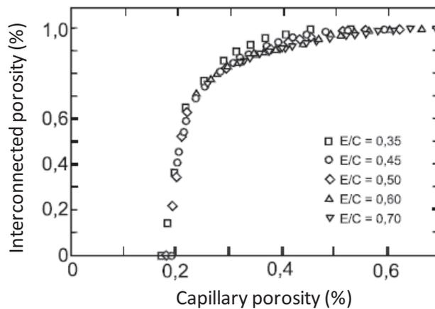
**Figure 2:** Evolution of the fraction of interconnected porosity vs the fraction of capillary porosity (Bentz and Garboczy, 1991).
