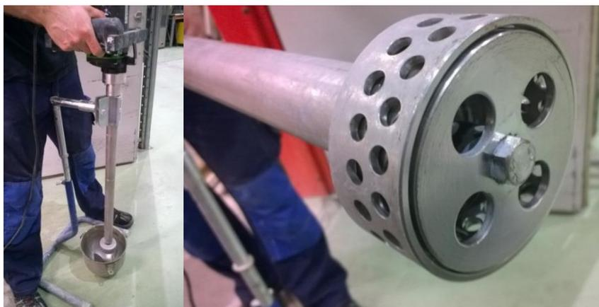
**Figure 4:** *High-speed mixer Desoi AKM-70.*
