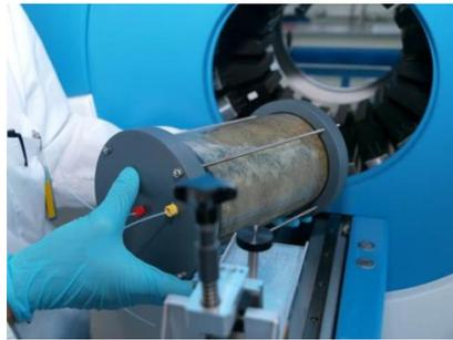
**Figure 1:** Typical sample for visualization of tracer flow with GeoPET.
