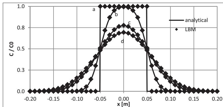
**Figure 3:** Comparison of LBM diffusive transport results (dots) to analytical solution (solid lines). Results for four time steps are conducted: a=0 s, b=166 667 s, c=858 333 s and d=1 216 667 s.
