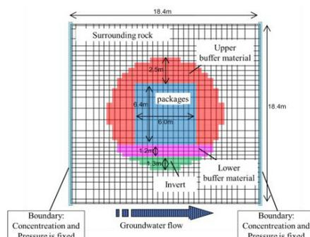
**Figure 2:** Geometry of the chemical-mass transport coupled calculation.
