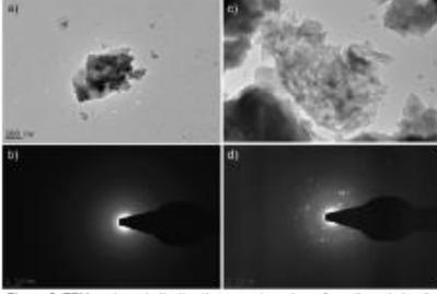
**Figure 5:** TEM analyses indicating the secondary-phase formations during the AFm-Cl-9.2 experiment. a) Electron micrograph showing the formation of an Al-rich phase. EDX analyses give a relative Ca:Al:Cl ratio of 0.5:1.4:0.1. b) SAED pattern showing the amorphous nature of the Al-rich phase. c) Electron micrograph showing a foil-like morphology. EDX analyses give a relative Ca:Al:Cl ratio of 1.0:1.0:0.0. d) SAED pattern showing the amorphous nature of the foil-like morphology.
