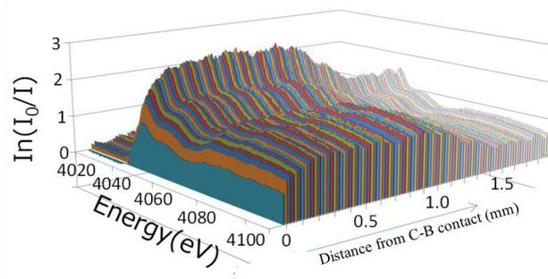
Figure 3: XANES spectra of bentonite around the cement-bentonite contact.
