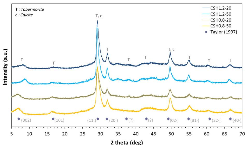
**Figure 2:** X-Ray powder diffraction spectra of synthesised dried C-S-H samples. For comparison purposes, data reported by Taylor (1997) for C-S-H(I) has been included. Letters stand for tobermorite (T) and calcite (c).
