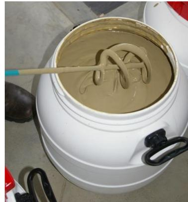
**Figure 2.** Preparation of bentonite suspension, at UJV.
