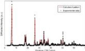
**Figure 2:** Experimental AFm-Cl XRD pattern (black crosses) and best fit to the data (solid red line).
