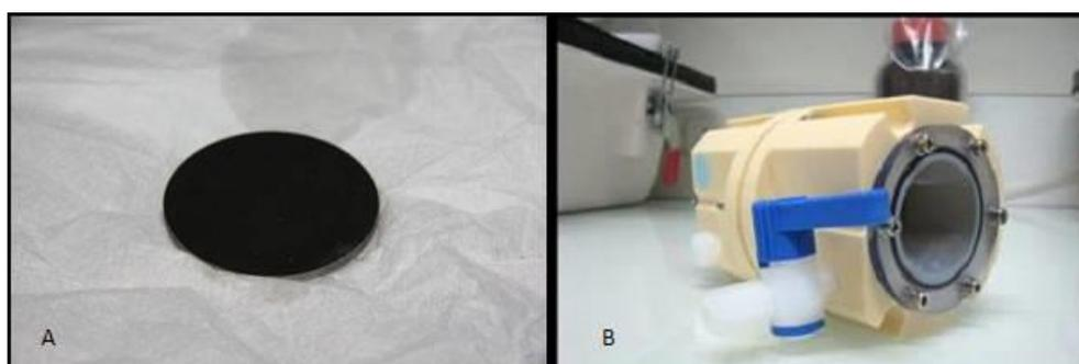
**Figure 13:** Classical diffusion cells used at Subatech (right) and sliced HCP.
