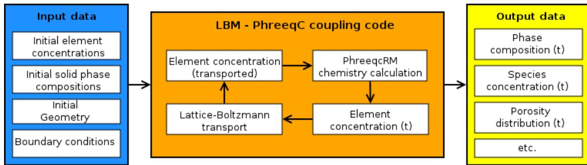
**Figure 1:** Calculation loop and data input/output scheme.
