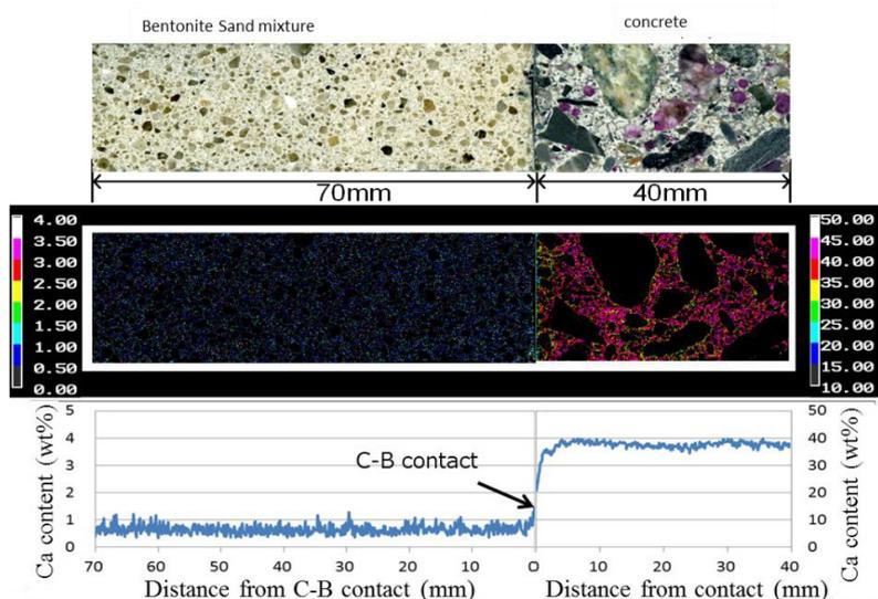
**Figure 2:** Results of the 2-D mapping of Ca-concentration around cement-bentonite contact.
