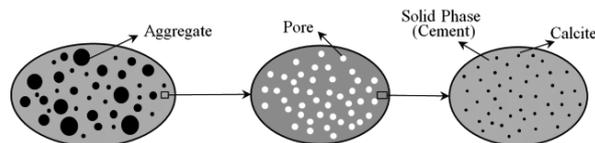
**Figure 1:** Representative volume element (RVE) of carbonated concrete.
