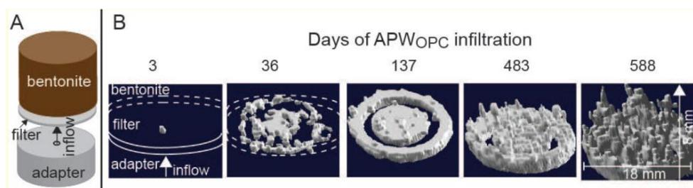
**Figure 5:** Time sequence of CT images taken with a medical tomograph over nearly 600 days of the interface region between compacted MX-80 bentonite and infiltrating high-pH fluid. A growing ring-shaped complex region of porosity plugging and mineral alteration is segmented from bentonite portions that did not change significantly in X-ray absorbance. Modified from Dolder et al. (2014).
