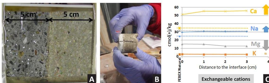
**Figure 2:** *A.* Example of aged (13y) shotcrete/bentonite specimen obtained by overcoring (March '15). *B.* Example of aged (13y) shotcrete/bentonite specimen obtained by dry drilling with a diamond coring machine (May '15). Samples are shared by UAM and CIEMAT teams. *C.* Example of variations of cation exchange population in one of the dry drilled cores.
