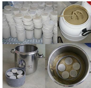
Laboratory procedures: cementitious thin plates and bentonite suspension
