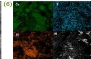
SEM imaging and EDX analysis (Figs. 5 & 6) confirmed the presence of the same phases identified by XRD and TG-MS: (A) Portlandite; (B) C-S-H; (C) ettringite; and (D) monocarboaluminate hydrate.
