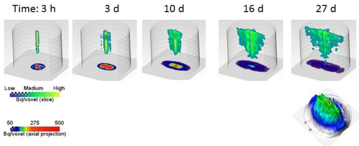
**Figure 4:** PET of diffusion of  $^{22}\text{Na}$  from a central drill hole in a 100 mm diameter Opalinus Clay core (from Kulenkampff et al., 2015). The central drill hole was filled with synthetic Opalinus Clay pore water, labelled with  $^{22}\text{Na}$ . Time frames: 3 h, 10 d, 16 d, 27 d after injection. The experiment continued over a period of more than 100 d. **Below:** axial projection showing anisotropy and heterogeneous effects of the last frame.
