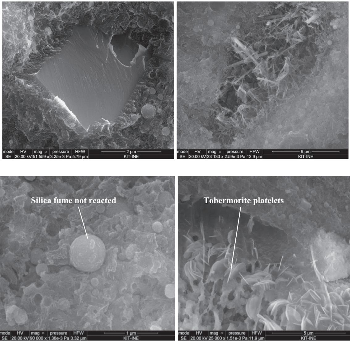
**Figure 6:** SEM pictures of mix 3C (**top-left:** presence of calcite, **top-right:** C-S-H phases, **bottom-left:** silica fume not reacted, **bottom- right:** tobermorite platelets).
