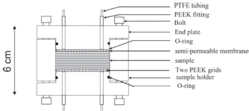
**Figure 7:** Schematic cross-section of a modified through-diffusion cell (Savoie et al., 2010).
