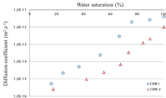
**Figure 5:** Evolution of diffusion coefficient vs water saturation for CEM I ( $w/c=0.4$ ) and CEM V ( $w/c=0.43$ ) concretes (Bourbon, 2013).
