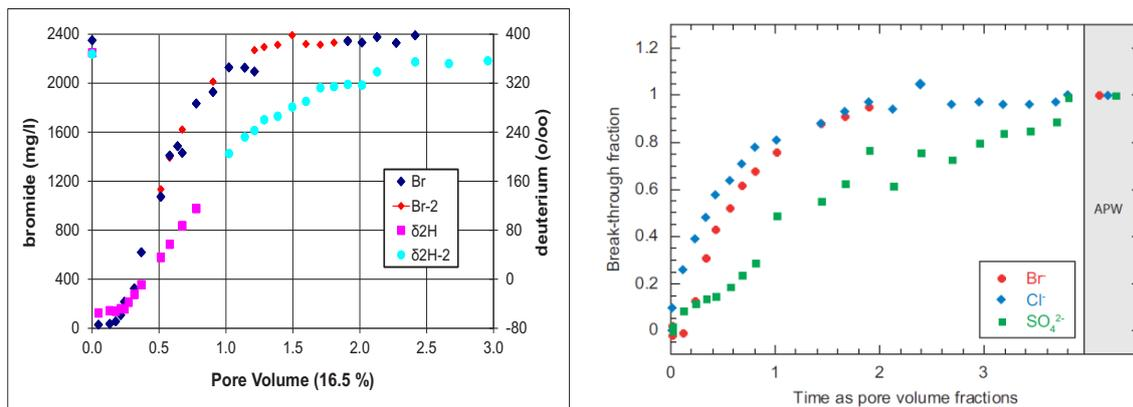
**Figure 4:** *Left:* breakthrough of water vs. bromide in a core infiltration experiment with Opalinus Clay from Mont Terri (Mäder et al., 2004), illustrating the anion-exclusion effect. Composition of APW is plotted at time zero. **Right:** small difference in anion transport between bromide and chloride, in comparison to sulphate that is controlled by reaction with a sulphate phase. Pore volume fraction is based on total water content.
