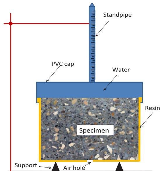
**Figure 6:** Schematic experimental setup to measure water sorptivity.
