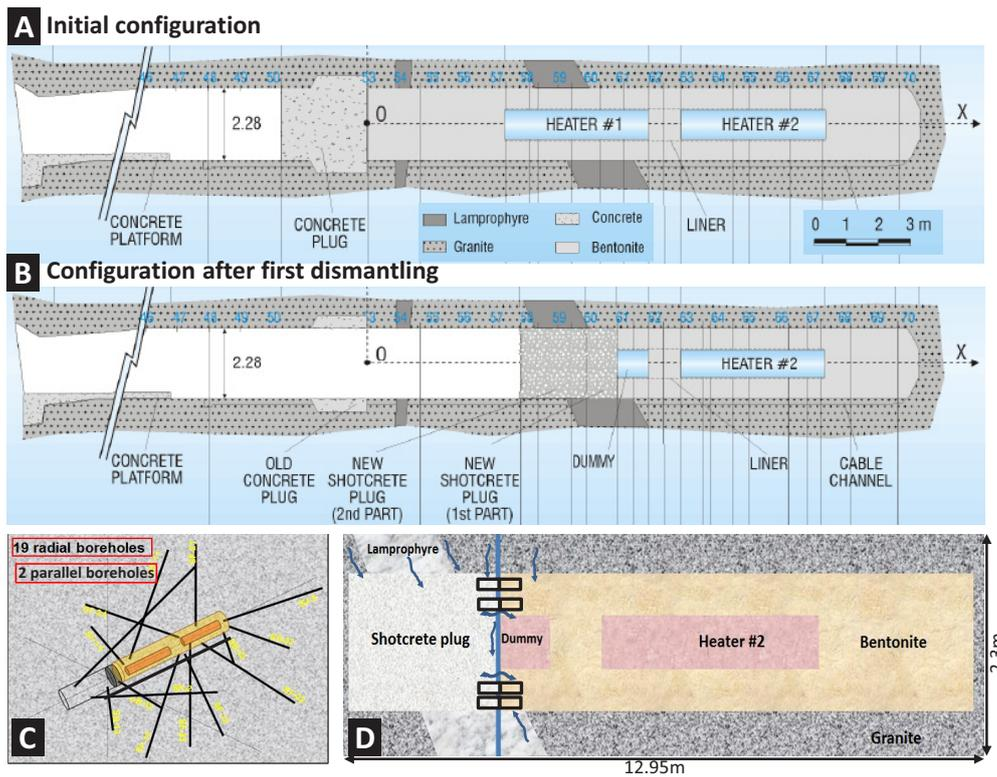
**Figure 1:** *A. Initial configuration of the FEBEX experiment. It was in operation for 5 years (1995-2002). B. Configuration of the FEBEX experiments after the first dismantling. It was in operation until 2015, when the experiment was completely dismantled. C. Location of boreholes for groundwater sampling around the FEBEX gallery. D. Simplified picture showing sampling position (rectangles) and water fluxes under consideration.*
