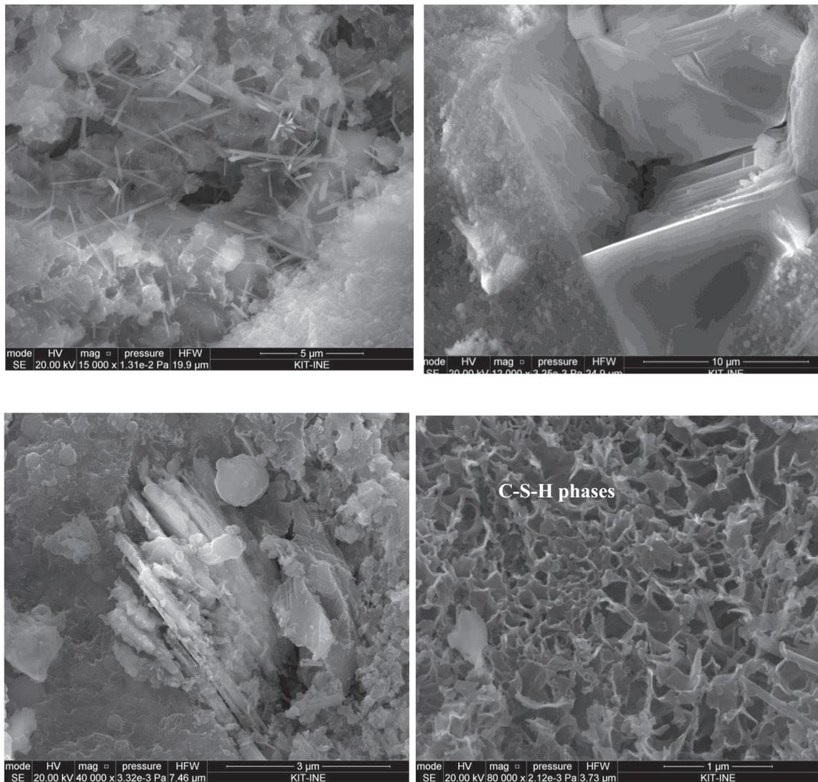
**Figure 7:** SEM pictures of mix 3D (upper row) and mix 3E (lower row) (**top-left:** crystalline C-S-H phases of tobermorite-type structure, **top-right:** presence of calcite, **bottom-left:** silica fume not reacted and calcite, **bottom-right:** C-S-H phases).
