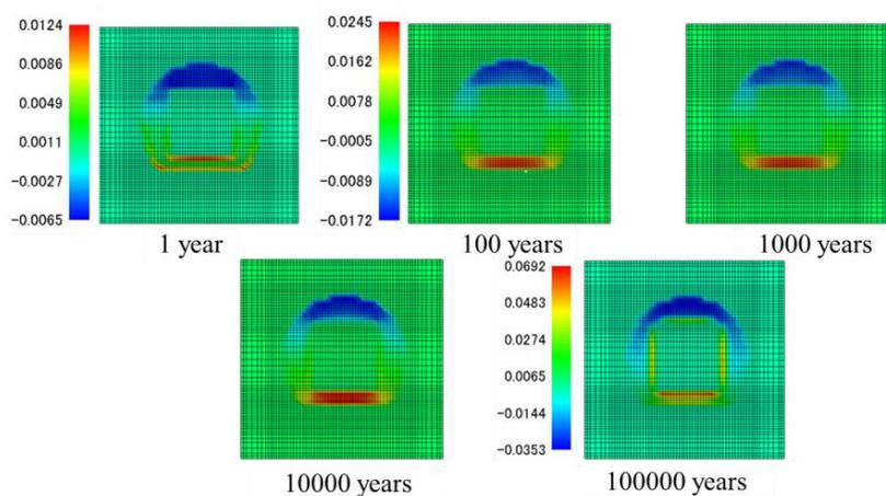
**Figure 6:** Distribution of volumetric stress in Case 3 for different times.
