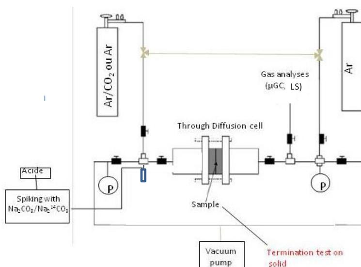
**Figure 14:** Sketch of the gas-diffusion set-up.
