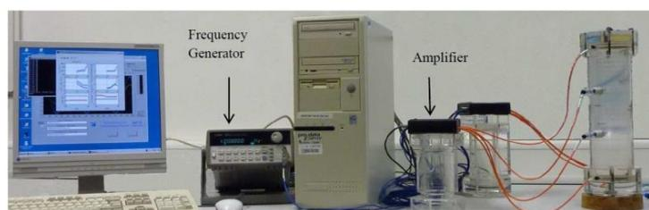
**Figure 2:** Sketch of the spectral induced polarization experiment.
