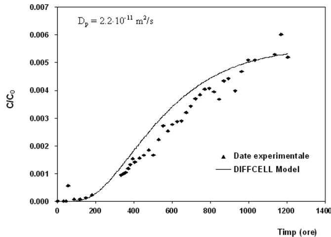
Figure 4: <sup>3</sup>H breakthrough curve and the theoretical one get for  $D_e = 2.2 \cdot 10^{-11} \text{ m}^2/\text{s}$ .
