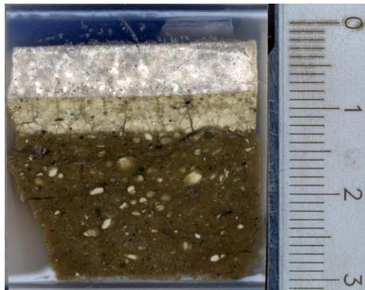
**Figure 3.** Example of investigation of aged concrete-bentonite interface within a concrete plug in a granite gallery context (study by UAM).
