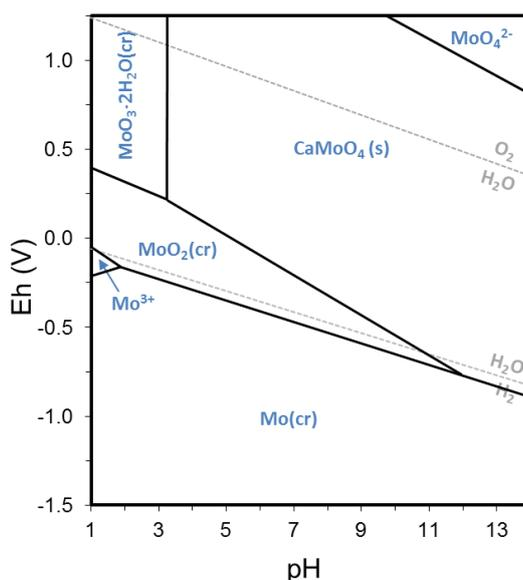
**Figure 1:** Predominance Eh/pH diagram of the system Mo-Ca-H<sub>2</sub>O at 25°C (Phase-controlled environment) [ $\text{Ca(II)}]=10^{-2}$  M; [ $\text{Mo(VI)}]=10^{-3}$  M. (Diagrams calculated in the present work with Spana v3 using ThermoChimie database v.9b0 (<https://www.thermochimie-tdb.com>)).
