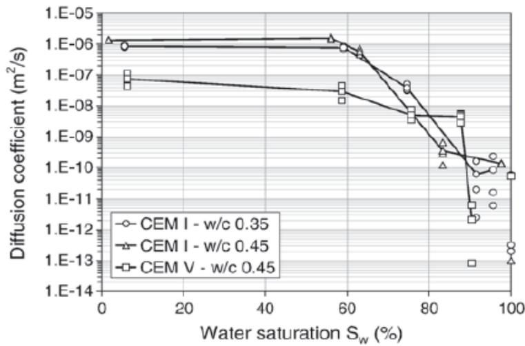
**Figure 12:** Hydrogen diffusion coefficient vs water saturation for CEM I ( $w/c = 0.35$  and  $0.45$ ) and CEM V ( $w/c = 0.45$ ) cement paste (Sercombe, 2007).
