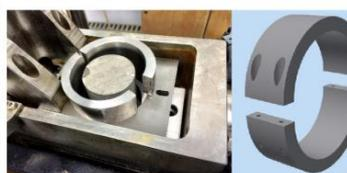
Effort in Year 1 has concentrated on equipment modification to allow 24 tests to be conducted using cylindrical samples
