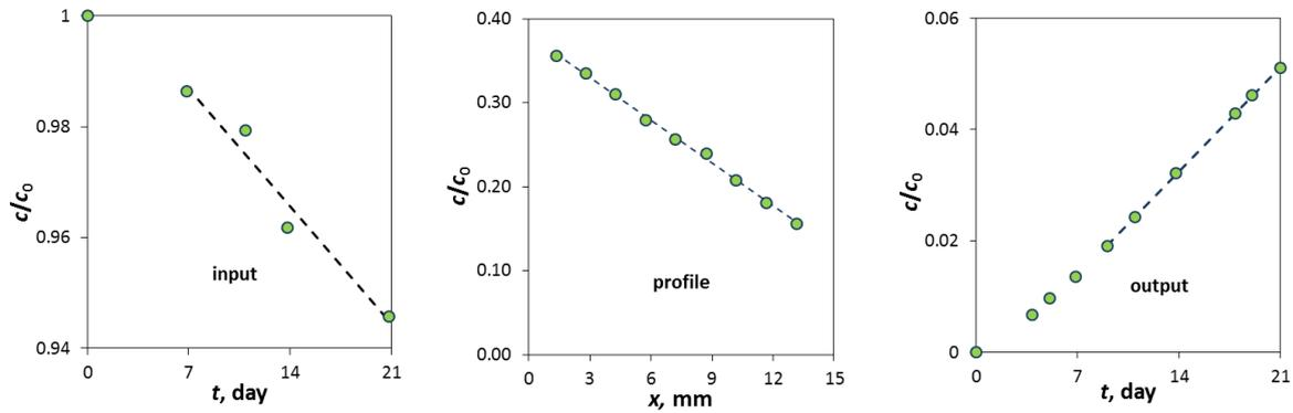
**Figure 1:** Illustration of the application of the method-of-lines for the evaluation of a real through diffusion experiment (diffusion of HTO through compacted bentonite) performed in the apparatus in which concentrations in working reservoirs are not kept constant.
