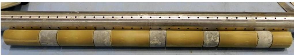
**Figure 2:** Cartridges: bentonite and cementitious samples preparation for placing into cartridge for in-situ experiment (2010).
