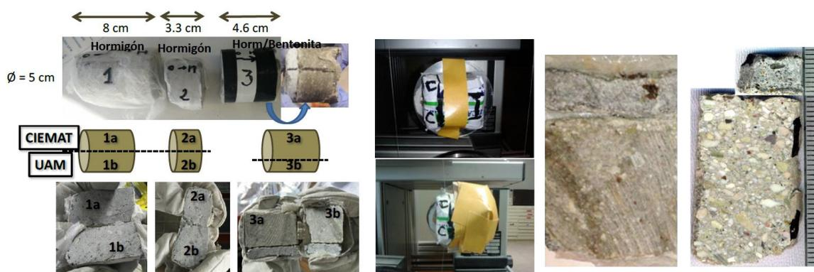
**Figure 2:** Sequence of cutting and preparation of in-situ interface taken samples shared with the CIEMAT team.
