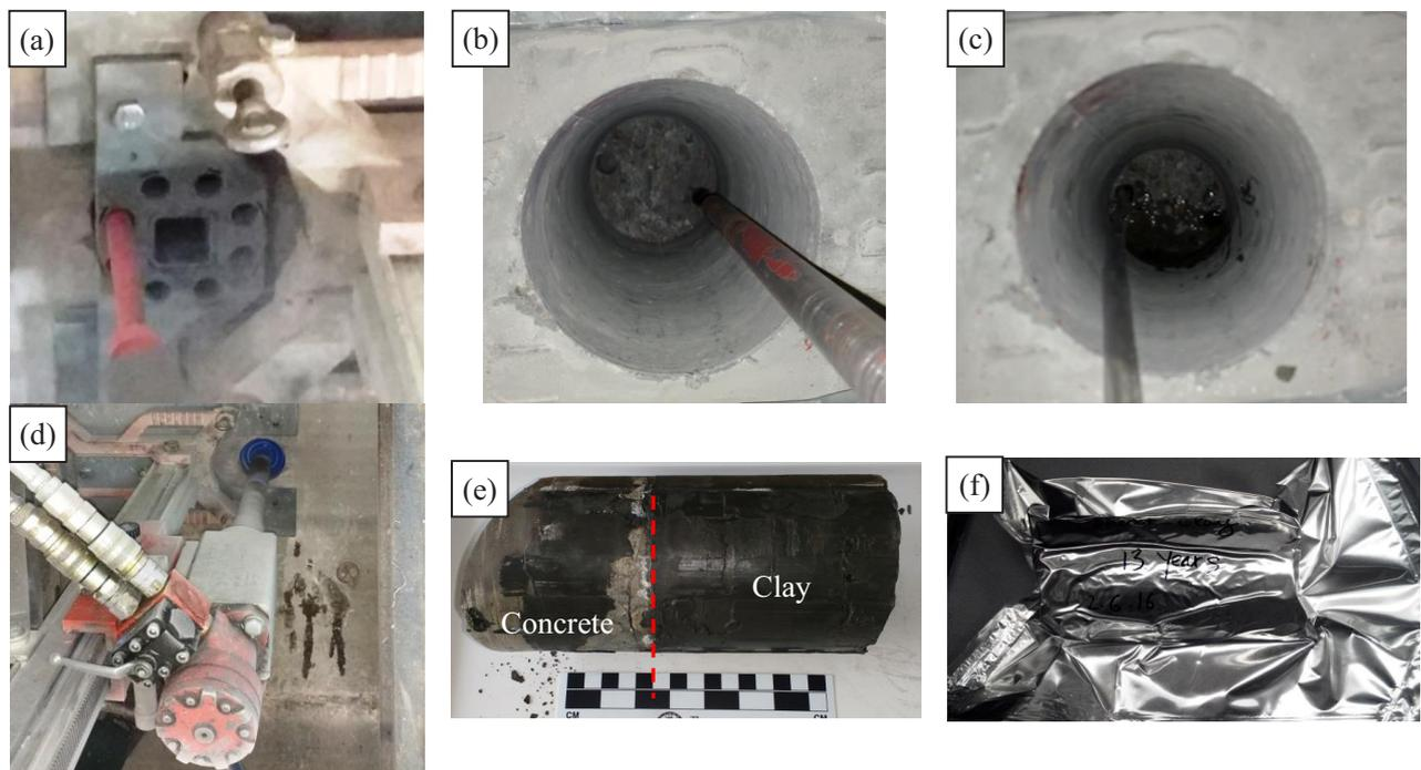
**Figure 2:** In-situ drilling procedure: (a) Drilling small hole using guiding system; (b) Two small holes for resin filling; (c) Resin filling into two small holes to make two anchors after polymerization; (d) Dry drilling concrete-clay interface after reinforcing by anchors; (e) Concrete-clay interface sample after retrieving from drilling bit; and (f) Sample packaged in aluminium foil.
