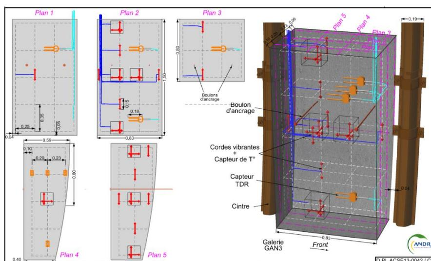
**Figure 4:** Thick wall geometry and monitoring device implementation.
