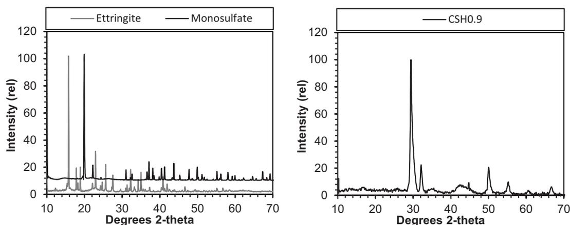
**Figure 1:** XRD pattern of the synthesized ettringite, monosulfate and CSH 0.9.
