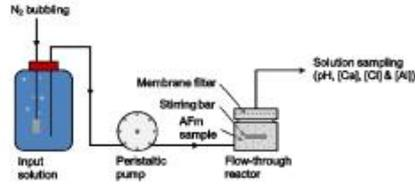
**Figure 1:** The experimental apparatus
