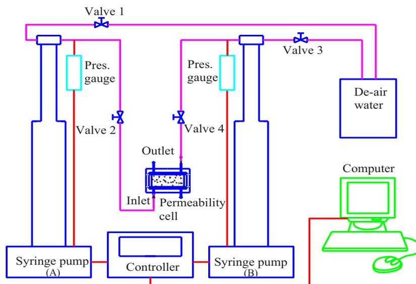
**Figure 4:** Schematic test setup for permeability determination.
