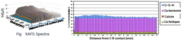
Fig. Results of the quantification of Ca-containing minerals by pattern fitting method
