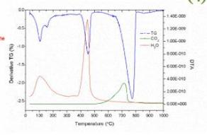
The main phases in the highly crystalline hydrate product assemblage were determined by XRD (Fig. 3) as calcite (CaCO<sub>3</sub>), portlandite [Ca(OH)<sub>2</sub>], ettringite (AFt phase) and monocarboaluminate hydrate (AFm phase). TG-MS (Fig. 4) confirmed these phases; two peaks between 100 and 300 °C correspond to ettringite and monocarboaluminate hydrate, while peaks between 400 to 500 °C, and 650 to 800 °C are related to Portlandite and calcite, respectively.
