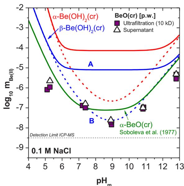
**Figure 1:** Solubility of Be(II) in 0.1 M NaCl. Symbols: experimental data obtained in the present work. Solid/dashed lines: thermodynamically calculated solubility of  $\alpha$ -BeO(cr),  $\beta$ -Be(OH)<sub>2</sub>(cr) and  $\alpha$ -Be(OH)<sub>2</sub>(cr) (see text).
