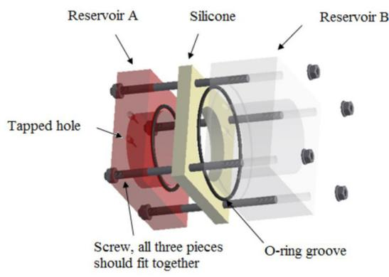
**Figure 3:** Flow-through diffusion cell.
