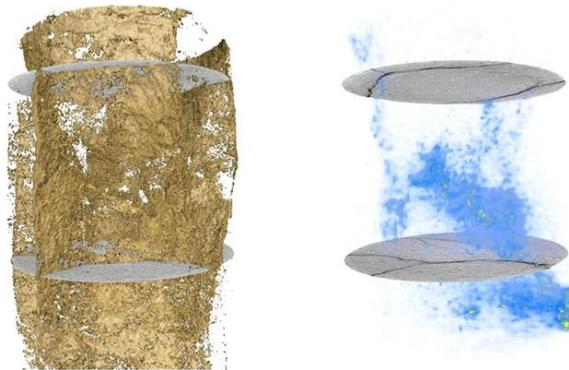
**Figure 2:** Different information provided by  $\mu$ CT and PET in a sample showing preferential pathways. **Right:** fracture surface from  $\mu$ CT-imaging, **left:** tracer concentration  $c_{PET}(x,y,z)$  from one PET-frame during flow experiment.
