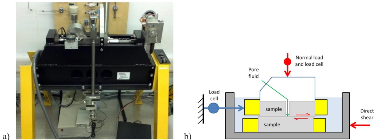
**Figure 1:** The direct shear rig (a) photo of the rig, (b) schematic of the apparatus.
