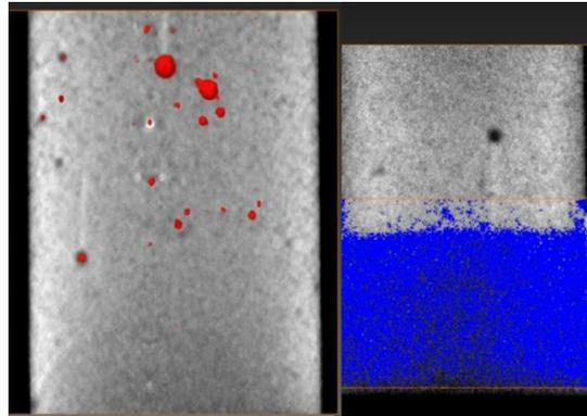
**Figure 2:** Neutron imaging of dried foamed concrete ( $\phi$  30 × 50 mm) -**left**- (the red spots represent the voids in the concrete) and absorbed  $D_2O$  (blue) -**right**- into the foamed concrete.
