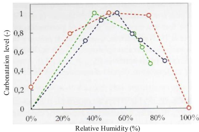
**Figure 1:** Evolution of the carbonation level vs relative humidity for different cement materials (from (Auroy, 2015 and references herein): red (Verbeck et al., 1958), blue (Papadakis et al., 1991), green (Thiery et al., 2005).
