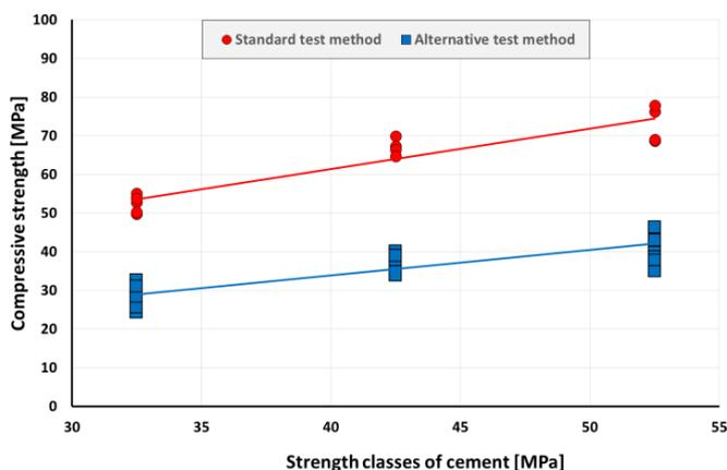
**Figure 3:** Comparison of two methods for testing of compressive strength of cement paste ( $w = 0.45$ ): standard test method (cubes  $40 \times 40 \times 40$  mm) – red colour and alternative method - thin plates with diameter of 50 mm and height of 8.2 mm – blue colour.
