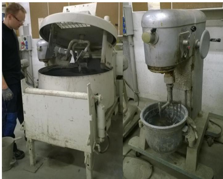
**Figure 3:** *Left: Zyklus mixer for concrete, Right: Hobart H400 mixer for paste.*
