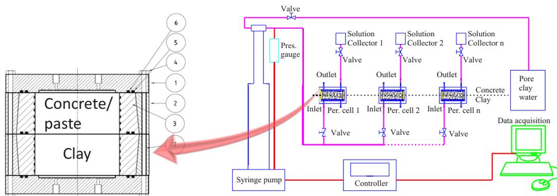
**Figure 3:** Schematic test setup for percolation experiment – the percolation cell (**left**) composes (1) steel lid, (2) steel body, (3) inner polycarbonate body, (4) bolt, (5) inner O-ring, (6) outer O-ring, and (7) threaded rod.
