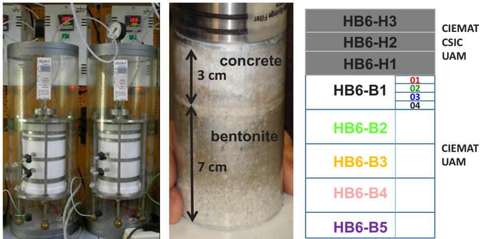
**Figure 3:** *Left.* Picture of the medium cells used for the study of the interfaces in the laboratory. *Centre.* Picture showing the aspect of the material once one of the cells was dismantled. *Right.* Sample distribution after dismantling of the HB6 cell (10 y of operation).
