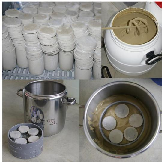
**Figure 1:** Laboratory procedures: cementitious thin plates and bentonite suspension.
