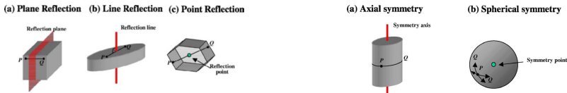
Figure 2.17: Different kinds of symmetry that exist in 3D space (from [Thrun and Wegbreit, 2005]).
