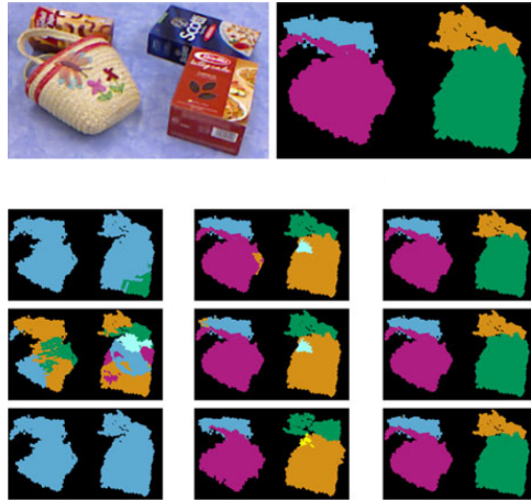
Figure 2.12: Top: Input image and ground truth. Bottom: Segmentations as estimated by three different samples from the probability distribution after 0, 5, and 15 pushes (from [van Hoof et al., 2014]).
