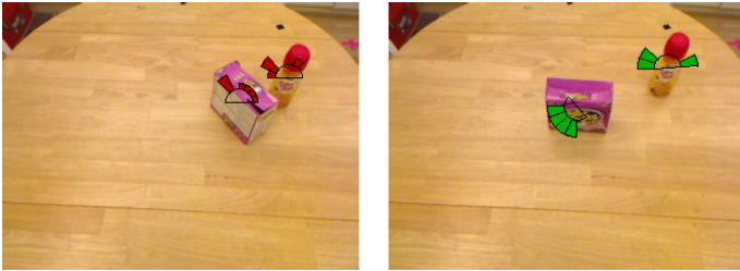
Figure 2.10: Left: Histogram of candidate boundary edge orientations. Right: Accumulated push history (from [Hermans et al., 2012]).
