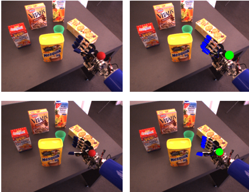
Figure 5.2: Localization of the hand of the robot, and in particular the fingertips, during grasping.
