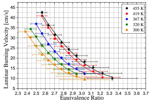
**Figure 5: Laminar burning velocities of Fuel-rich methane oxygen mixtures at different preheating temperatures and ambient pressure**
