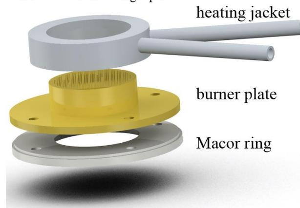
**Figure 2: Parts of the burner head**
