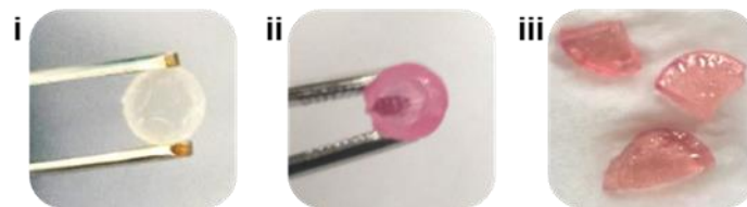
Figure 10 Display of a degradable network based on 99.8 wt.% DiHDA-linker + 0.2 wt.% Ivocerin®. At 25 °C, the network is rigid and not bendable (i). At 100 °C, the network can easily be bend by using tweezers (ii) and cut into pieces (iii).
