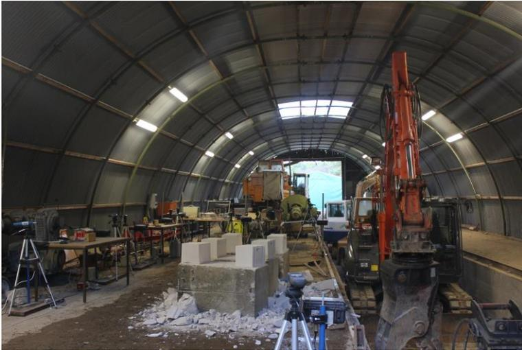
**Figure 5-16: Setup of the first experimental series: equipment (right side), masonry stones on blocks (in the middle) and measurement systems (left side, in the back, and at the front in the middle)**
