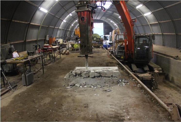
**Figure 5-17: Setup of the second experimental series for mortising: equipment (right side), concrete block on a concrete plate (in the middle) and measurement systems (left side and at the back)**
