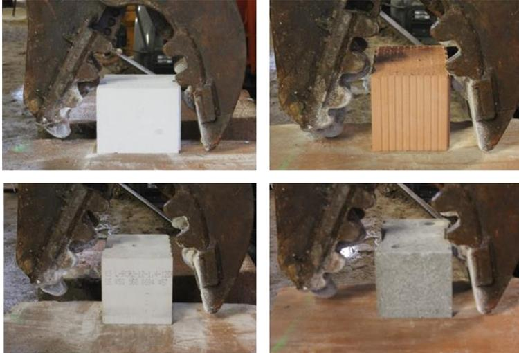
**Figure 5-19: Explored masonry stones made out of aerated concrete (top left), brick (top right), sand lime brick (bottom left) and concrete (bottom right)**
