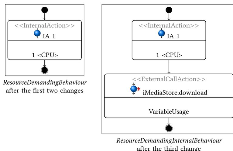
Figure 4.13.: The resulting *ResourceDemandingInternalBehaviour* of the incremental SEFF creation from the `doDownload` method. On the left side the result after the first two changes is depicted. On the right side the result after the third change, which inserts the call to the `download` method of the `IMediaStore` interface, is depicted.
