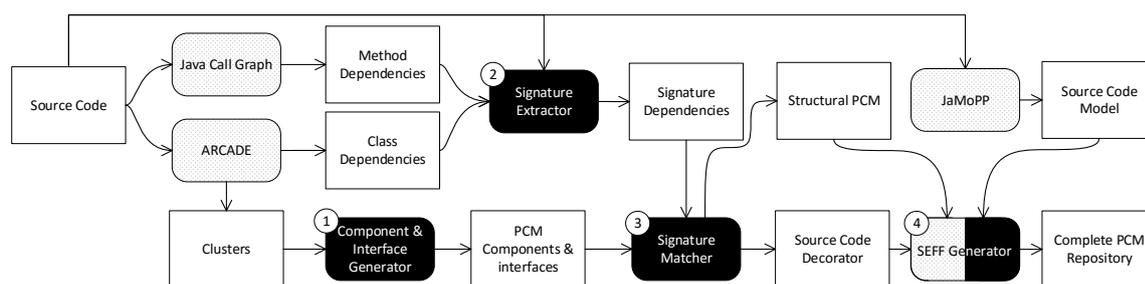
Figure 5.2.: Overview of architecture reconstruction approach *Extract*. We need to execute steps 1 through 4 to get a PCM instance from source code. The grey boxes, are approaches, we could reuse, while the black boxes are contributions of *Extract* (step 1 through 3). We were able to reuse SoMoX’s *SEFF* generator for *Extract*, but we need to adapt it in order to work in the environment of *Extract*.
