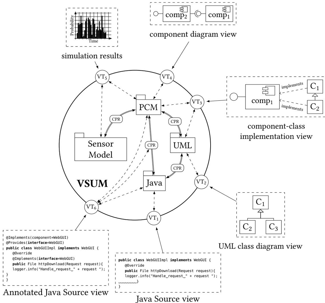
Figure 4.4.: The VITRUVIUS vision applied to the CBSE domain, as we [KBL13] and Burger [Bur14] proposed. As models we use the PCM, UML, the PCM Sensor Framework model, and a model of Java source code. The consistency preservation rules between the model instances are depicted as the arrows annotated with CPR. The view types are either combining view types (if they contain information from more than one metamodel) or projectional view types (if they contain information from one metamodel only).
