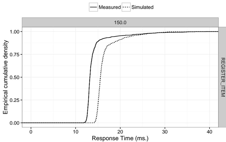
Figure 6.12.: Cumulative response time distribution of measurements compared to simulation results for the extracted model. The x-axis shows the response time in milliseconds. In the simulated run as well as in the measured run nearly all requests are processed within the first 25 ms. The mean interarrival time of new users is 150 ms.
