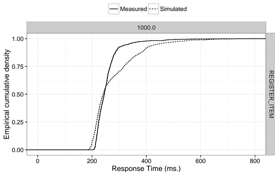
Figure 6.13.: Cumulative response time distribution of measurements compared to simulation results for the coevolved model. The x-axis shows the response time in milliseconds. The evolved system requires more time to process requests, i.e. most requests are processed within a range of 200 and 500 ms. The mean interarrival time of new users is 1000 ms.
