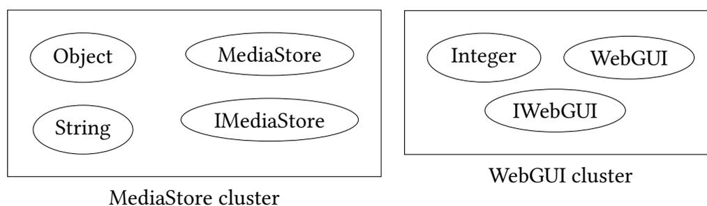
Figure 5.3.: Clusters of the MediaStore example extracted with ARCADE. We assume that two clusters are reverse-engineered by ARCADE. One cluster contains the MediaStore classes, while the other cluster contains the WebGUI classes.
