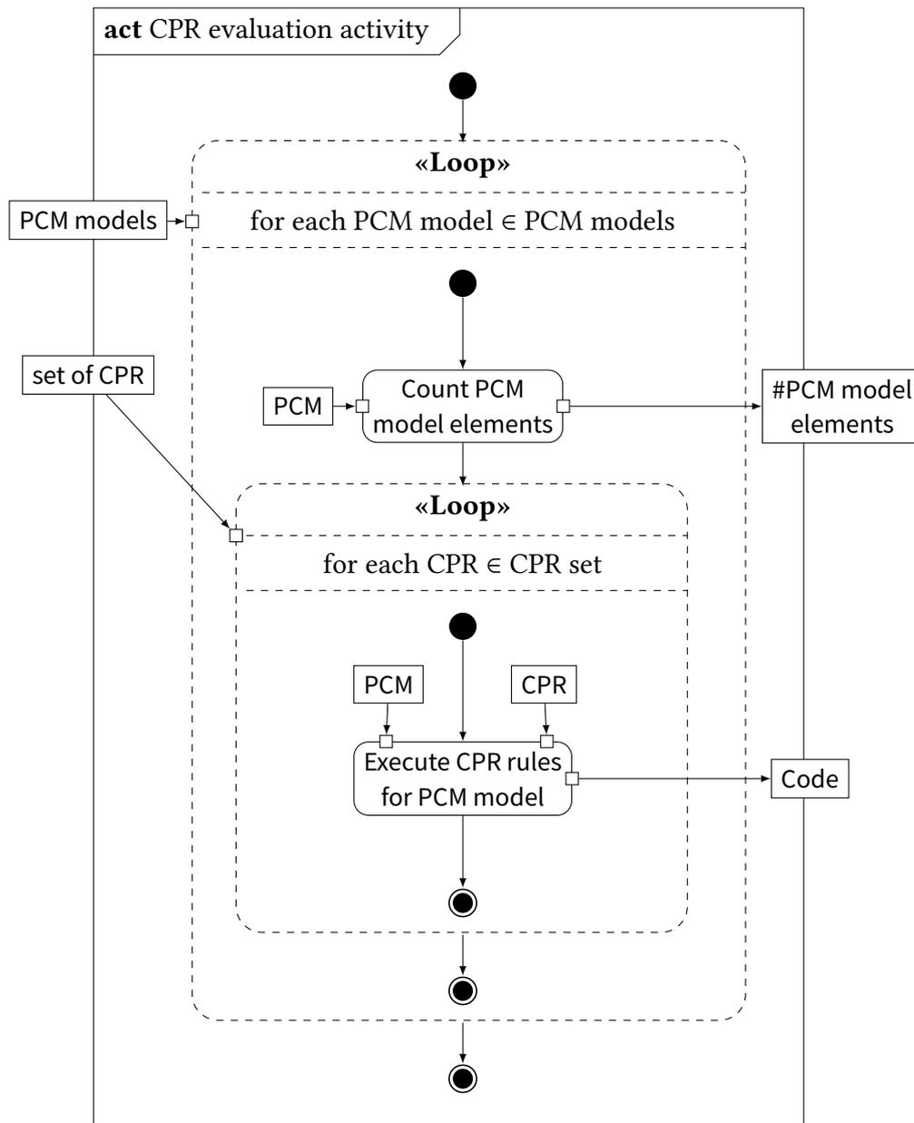
Figure 6.3.: Activity diagram of the evaluation helper tool. The tool applies a given set of consistency preservation rules to a given set of PCM models.
