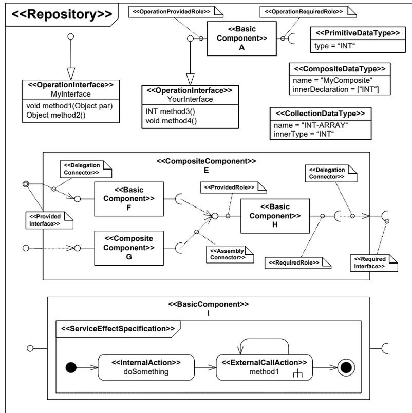
Figure 2.6.: Metaclasses in the PCM *Repository*[Reu+11], which are used within this thesis. The upper part depicts *BasicComponents* and *OperationInterfaces* and the relations between them. The middle part shows the internal structure of a *CompositeComponent*. The lower part shows a simple *SEFF* contained in a *BasicComponent*.
