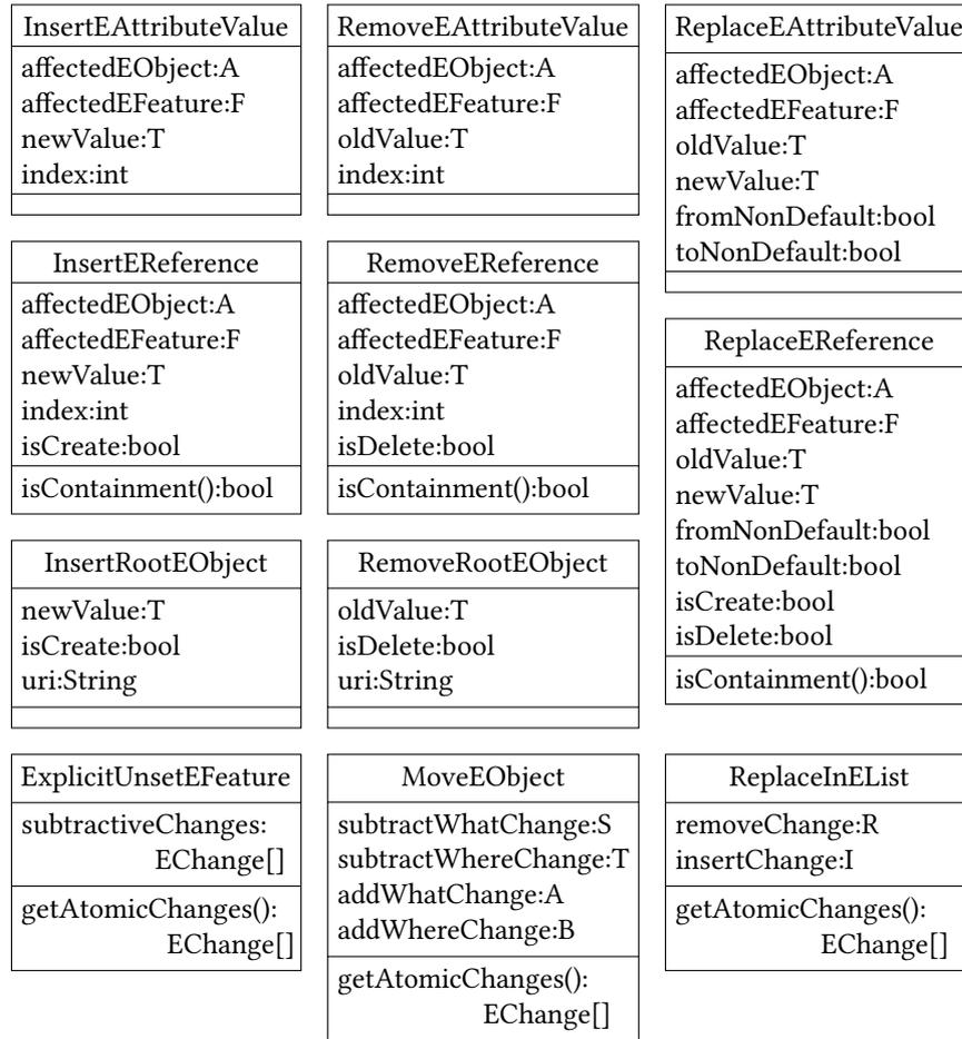
Figure 3.1.: Non-abstract, i.e, final classes of the change metamodel for VITRUVIUS ([Kra17]). Kramer [Kra17] presents a feature diagram for changes in EMOF and Ecore based metamodels and derived the change metamodel for VITRUVIUS from it. In the figure, we omitted the permute changes, because they are not supported yet. We have also simplified the name of the classes and omitted the type parameters.
