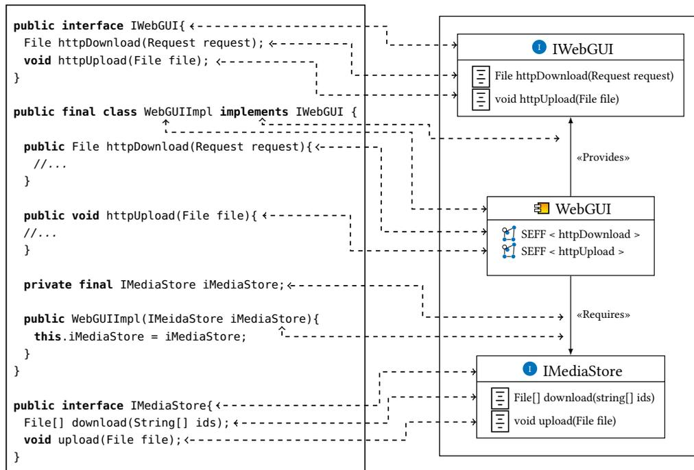
Figure 4.8.: The mapping between a *BasicComponent* and its provided and required *OperationInterfaces* to the corresponding source code elements using the package mapping consistency preservation rules
