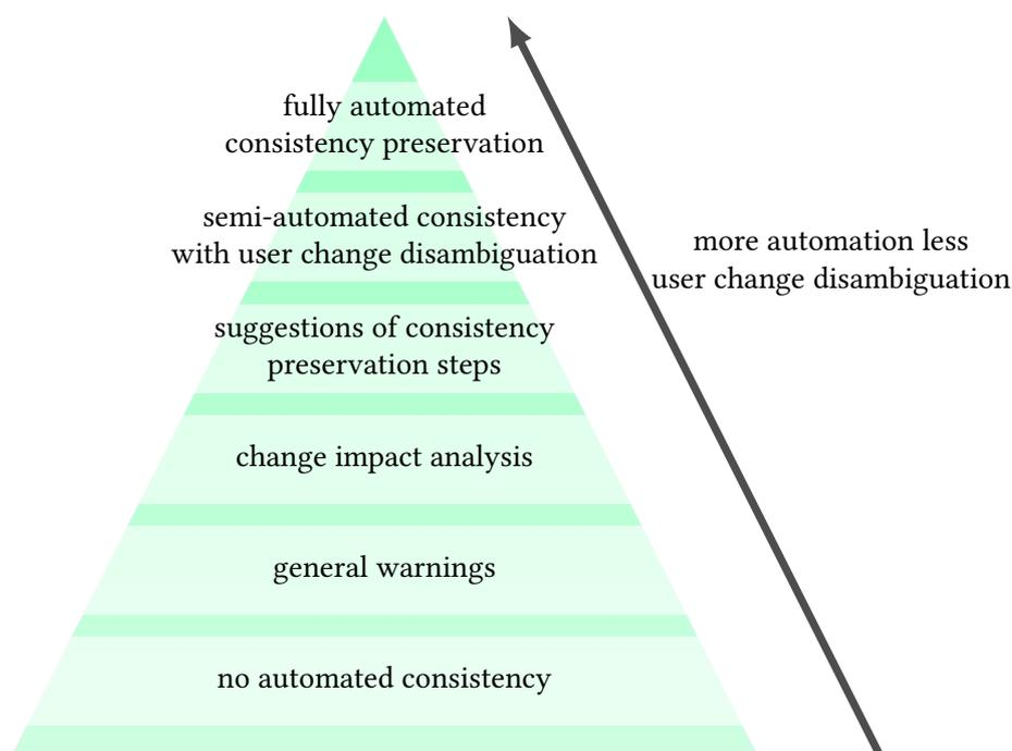
Figure 4.9.: Different levels of automation in VITRUVIUS for consistency preservation based on [Wer16] and [Kra17]. For our Coevolution approach only the top three levels are relevant.
