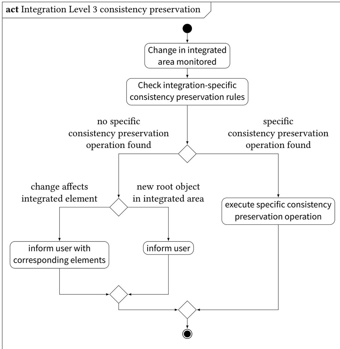
Figure 5.6.: Change processing in Integration Level 3. The figure shows the necessary steps if a change in an integrated area has been monitored. To simplify the figure, we did not include the standard VITRUVIUS case [Pet16].
