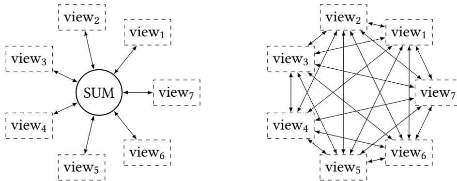
Figure 2.3.: Hub-and-Spoke approach vs. Peer-to-Peer approach [Bur14]
