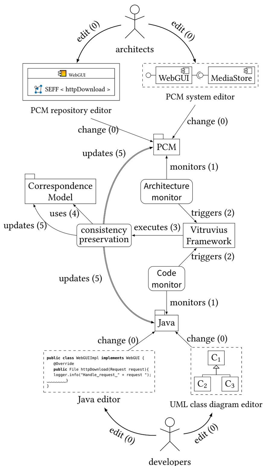
Figure 4.1.: The steps our Coevolution approach executes to keep architectural models consistent with the source code. Step zero (0) is performed by users of the architectural model editors or the source code editor. This step is not influenced or changed by our Coevolution approach. In reaction to step zero, however, our Coevolution approach performs the steps (1) through (5) in order to keep architectural models and the source code consistent.
