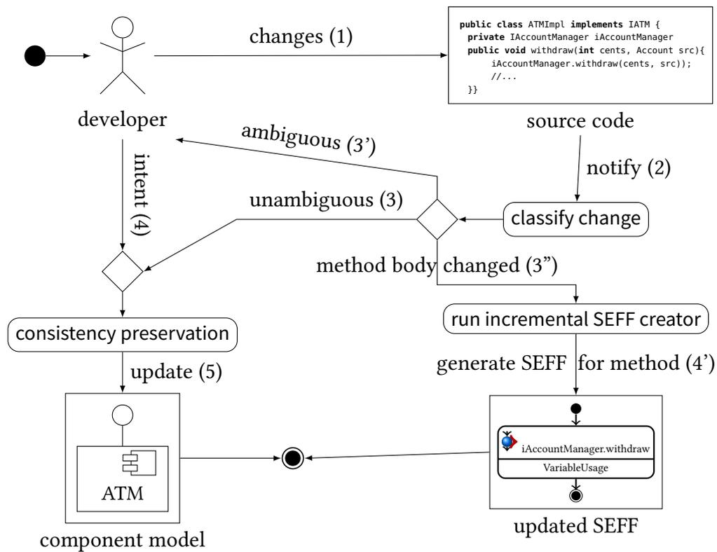
Figure 4.2.: The process how our Coevolution approach keeps source code changes consistent with the architectural model (see [LK14])
