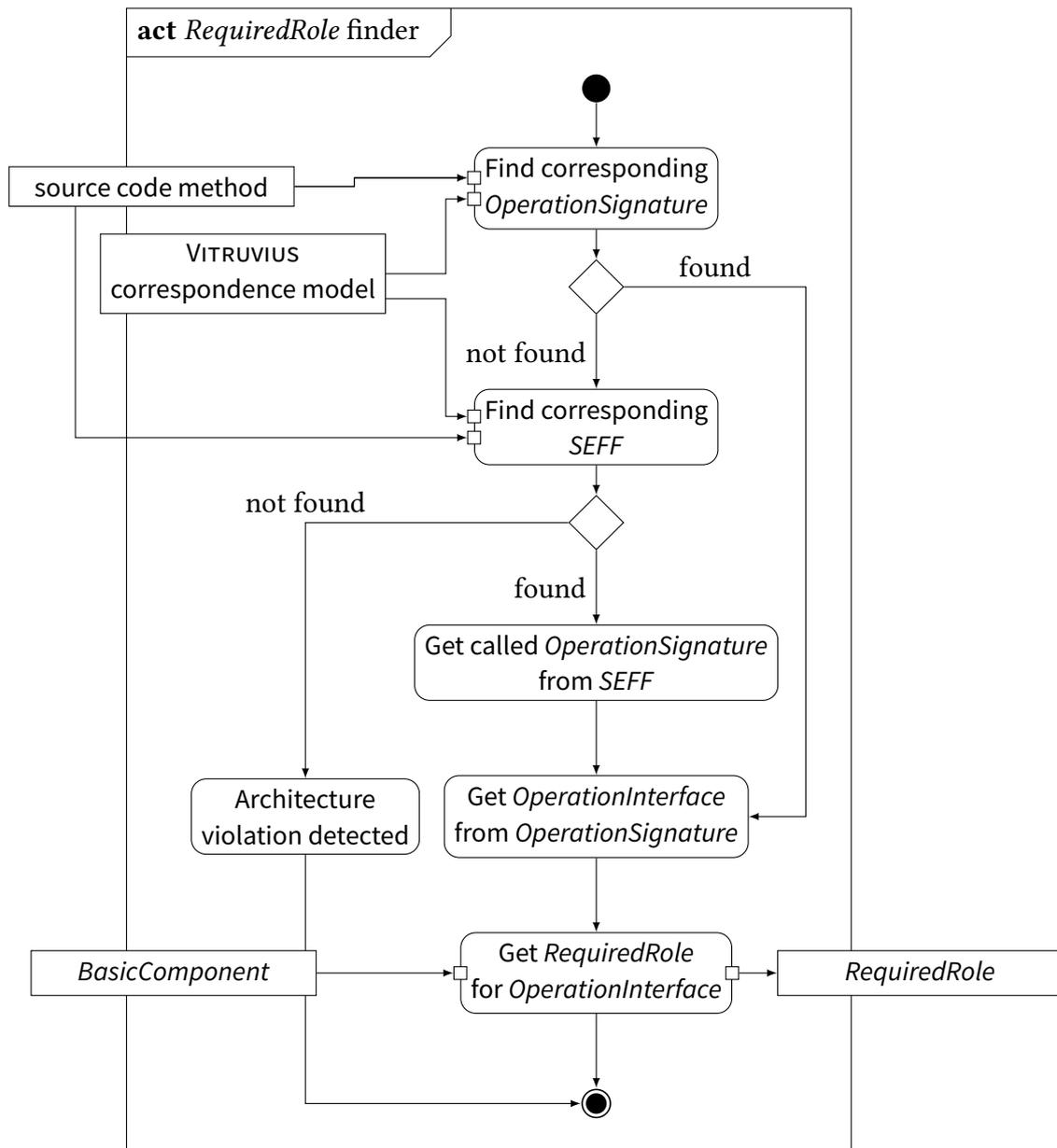
Figure 4.11.: Activity diagram that shows, how the *RequiredRole* finder for the package mapping consistency preservation rules is realised. The input for *RequiredRole* finder are the changed source code method, the VITRUVIUS correspondence model, and the current PCM *BasicComponent*. The output is the corresponding *RequiredRole*, which is used by the method call. We left out the object flow inside the activity diagram to simplify the diagram and improve its clarity.
