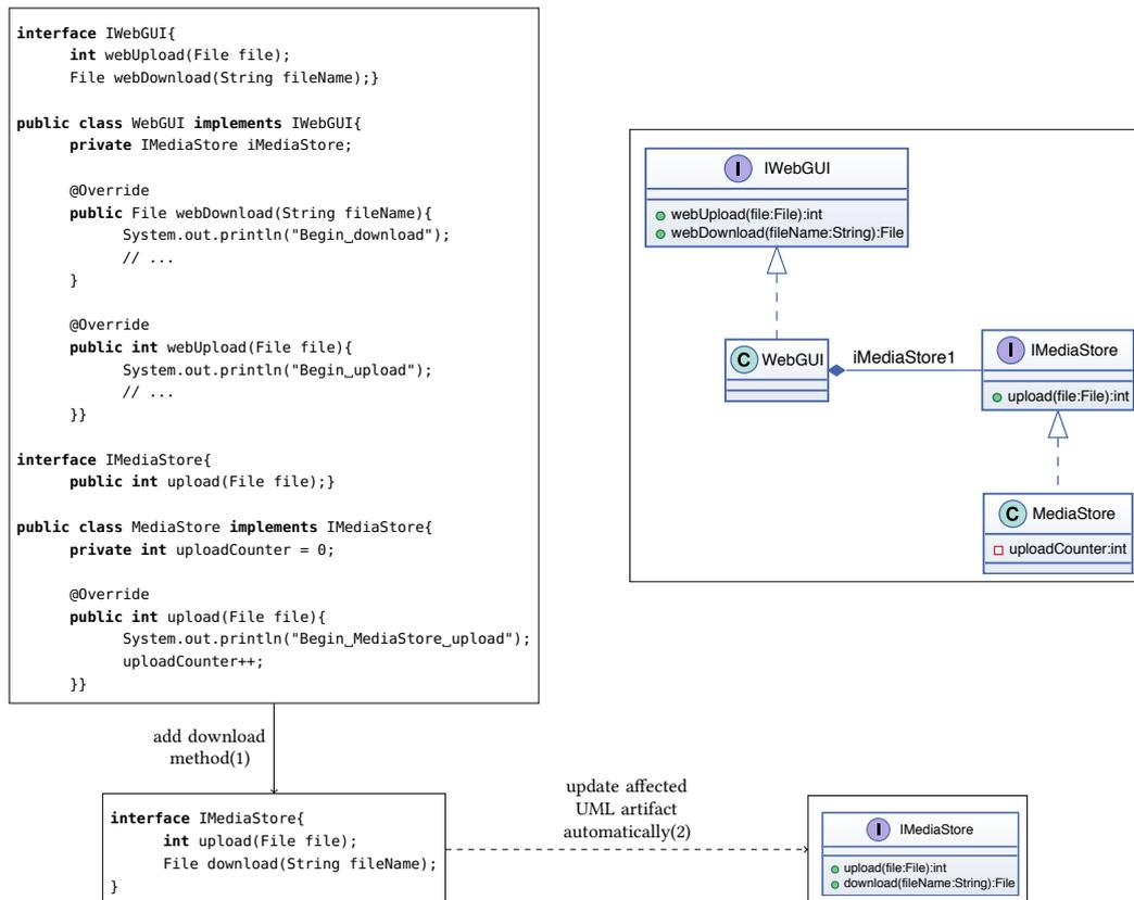
Figure 4.3.: The UML Class Diagram Editor applied to our running example [KLK16]. The left upper part shows the source code of the MediaStore. The right upper part shows the corresponding UML class diagram.
