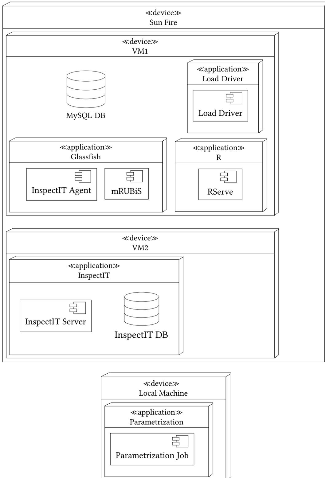
Figure 6.11.: Deployment diagram for the evaluation setup
