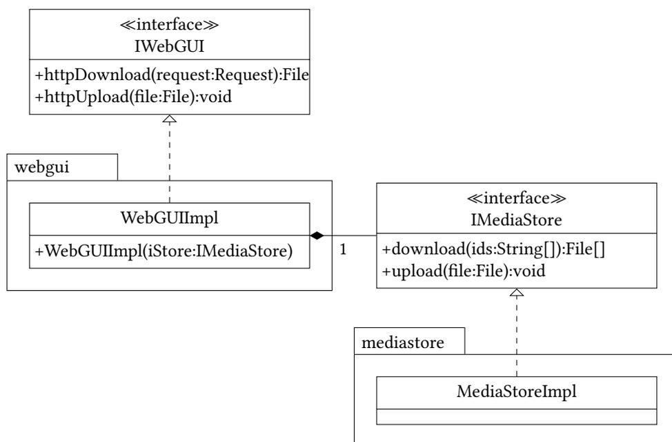
Figure 4.7.: The UML class diagram of the MediaStore example. To ease the diagram, we omitted the contracts, the repository, and the datatypes package.
