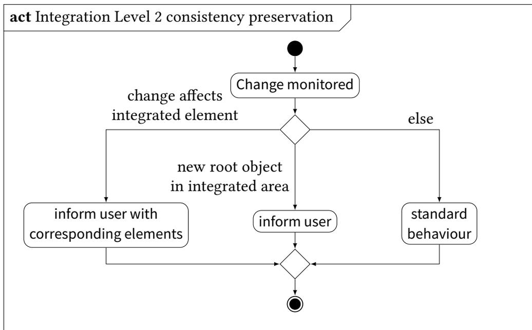
Figure 5.5.: Change processing in Integration Level 2. After we monitored a change, we check whether the change has been performed to an element within an integrated or not. In the first case, we need to inform users about the change (either with the corresponding element or without the corresponding element). In the latter case, we can use the standard consistency preservation rules can be used (standard behaviour)[Pet16].
