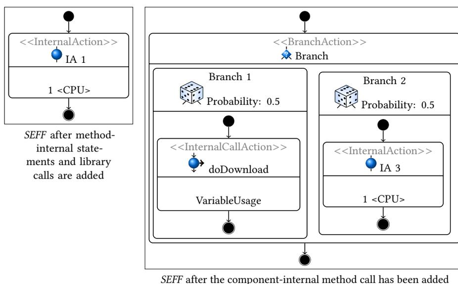
Figure 4.12.: The resulting *SEFF* of the incremental *SEFF* creation from the download method. On the left side the result after the first two changes is depicted. These changes introduce library calls or method internal statements only. The right side shows the result after the third change. This change introduces the component-internal method call to the `doDownload`.
