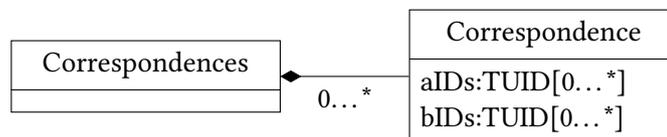
Figure 3.2.: The correspondence metamodel we used in the consistency preservation process. All actual Correspondence instances are contained in the root class Correspondences.
