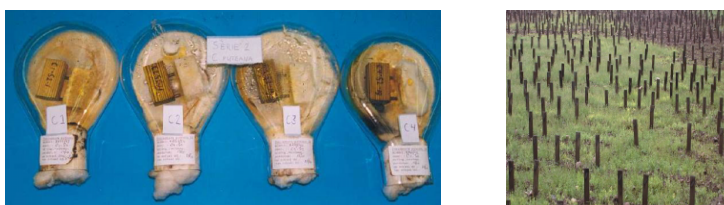
Figure B4-1 Left: Specimens in the laboratory in accordance with EN 113. Right: Outdoor test bodies in accordance with EN 252. (Rapp and Augusta, 2000)
