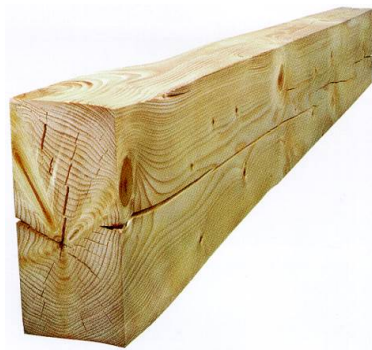
Figure B6-2 Squared timber with pith, knots and drying cracks. (Studiengemeinschaft Holzleimbau, 1998)
