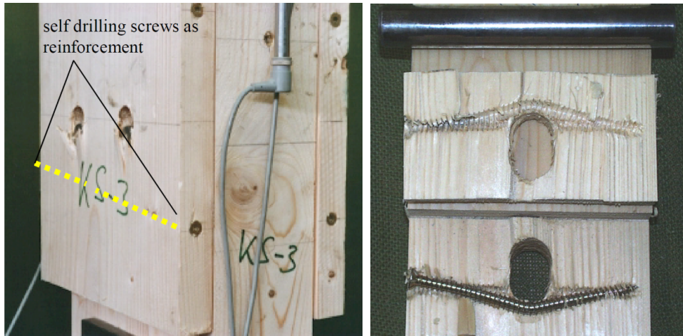
Figure E12-3 Joints reinforced with fully threaded screws. Left: reinforcement with a distance to the dowels. (Schmid, 2002) Right: opened specimen after test with reinforcement directly underneath the dowel. (Bejtka, 2005a)
