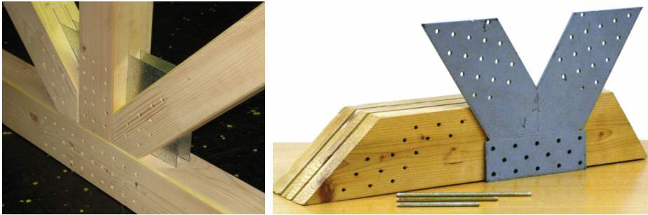
Figure E15-1 Left: GREIM system: truss joint between one post, two diagonals and lower chord, respectively made of glulam, nailed joint with two galvanized gusset plates. Right: connection BSB: slotted-in and predrilled glulam, galvanized predrilled 5 mm thick gusset plates and 6.3 mm thick dowels in lengths as required.
