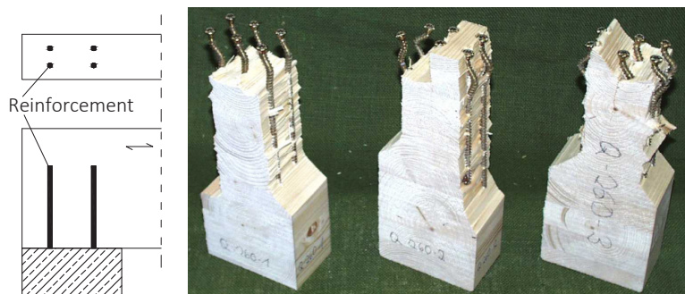
Figure E5-2 Left: Example of a reinforcement in a beam support. Right: Test specimens with buckled screws (Bejtka, 2005).
