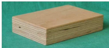
Figure B6-21 Laminated veneer lumber made of beech veneers.
