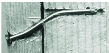
Figure E2-13 The nail is pulled out of the timber.
