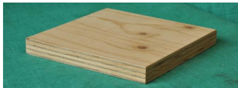
Figure B6-18 Plywood with longitudinal and perpendicular veneers of various thicknesses.
