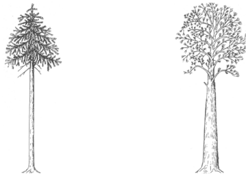
Figure B3-1 Stem shapes: left prismatic, right tapered. Tapering tends to occur; particularly in free-standing trees and at leeward forest areas. A significant decline in diameter to the smaller stem end (= tree taper) has a very detrimental effect on usability and yield. (Steuer, 1990)
