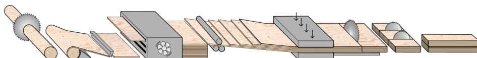
Figure B6-20 Production method for veneered materials. (Metsäwood, brochure „Ich bin Kerto“, 2014 version)
