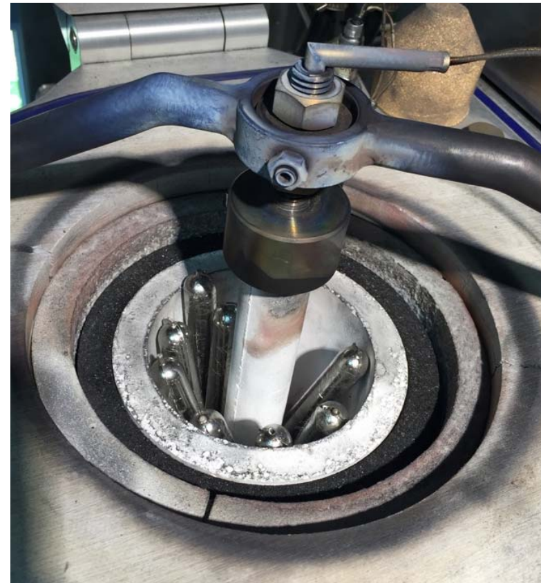
CoCrFeMnNi rods in a crucible of a vacuum induction furnace
