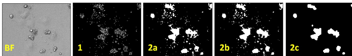
Figure 2.19: Channel B segmentation (steps 1-2 from Fig. 2.18): Channel B (section of original Channel B image taken from Benchmark dataset 2), 1 (edge detector), 2a (image closing), 2b (hole filling) and 2c (image opening).
