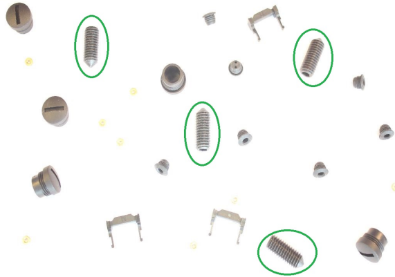
Figure 3.4: Using abstract ground truth information to find one targeted object in the scene. Set screws encircled in green are to be found in r = 1
