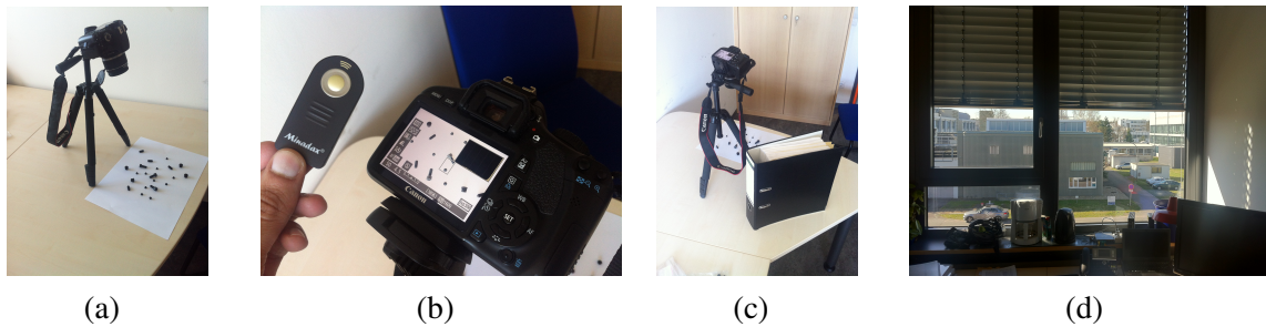
Figure 2.2: Experimental setup consisting of a professional camera mounted on a tripod with different objects placed on A3 white paper lying on the table (Fig. 2.2(a)), Remote camera trigger (Fig. 2.2(b)), use of paper documents folder for shadow construction (Fig. 2.2(c)) and Rolling window curtain (Fig. 2.2(d))
