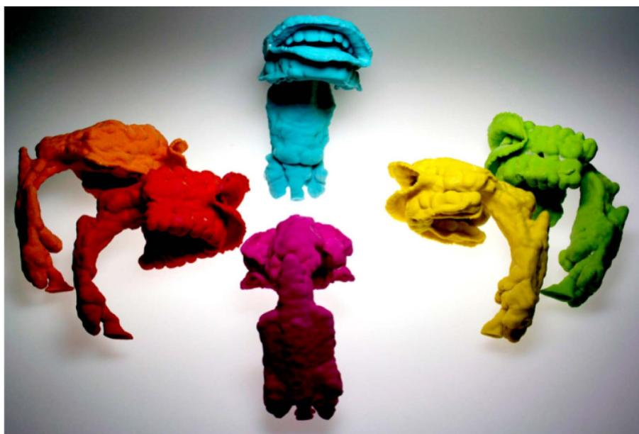
Fig. C.2 3D printouts of different phonations of the vocal tract acquired by MR imaging and printed with a powder printer.
