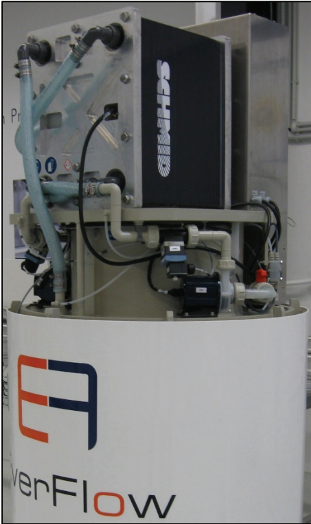
Figure 1-5: 2-kW/10-kWh VRFB prototype by SCHMID Energy Systems GmbH, Freudenstadt, Germany [10]
