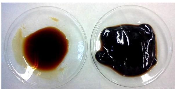
**Figure 3.1:** Light phase (left) and heavy phase (right) of a fast pyrolysis oil from wheat straw.
