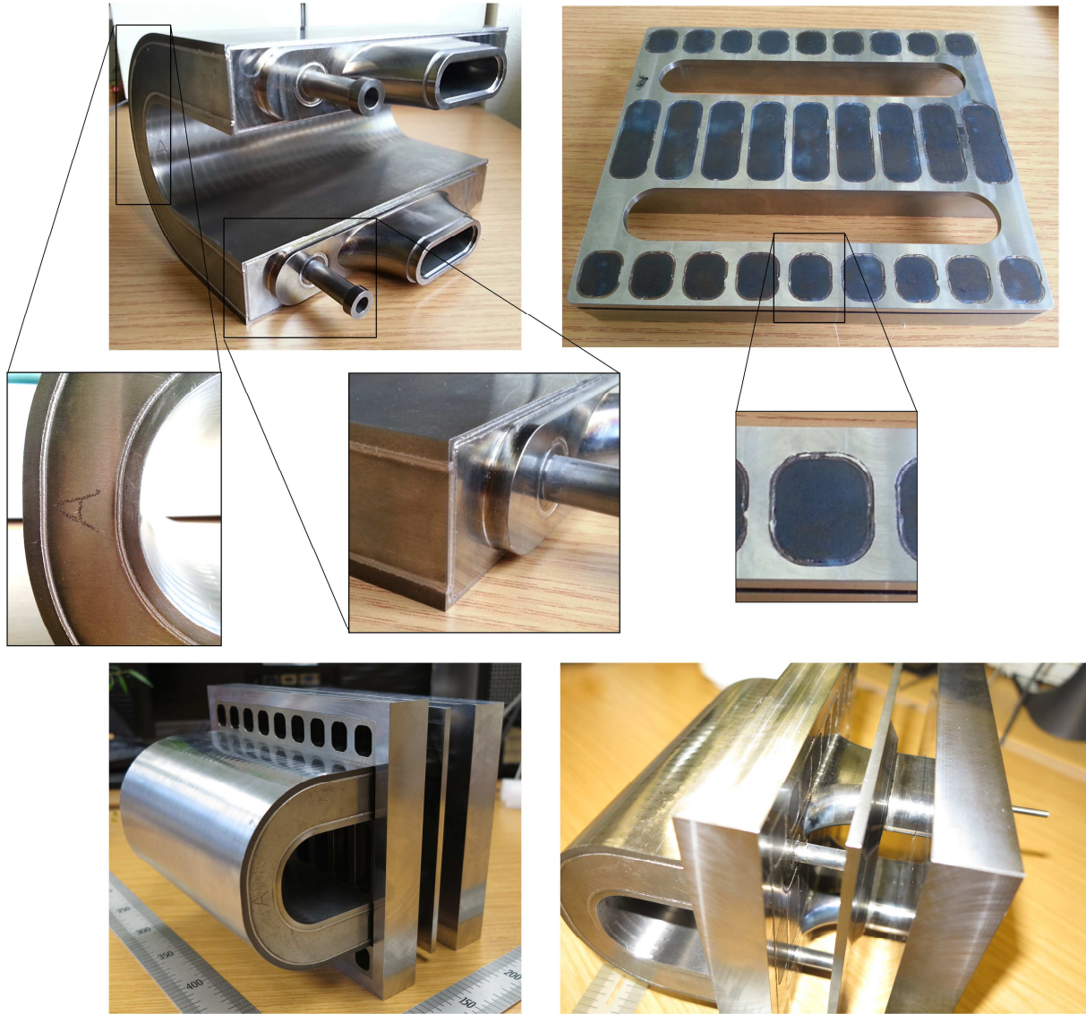
Figure A.5: Welding Group WG5 (top left) and WG6 (top right) with augmented views (middle) and finished assembly (bottom left and right). Despite the multiple sub-assemblies in WG7 or the multiple welding seams in WG6, the order of magnitude O of the distortions \delta is very low ( O(\delta) \approx 10^{-1} \text{ mm} ), allowing a successful assembly.
