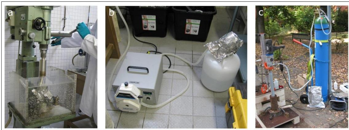
**Fig.9: Inner coring operations. a/b: Autoclaved distilled water was used for the preparation of the Exter Formation rock cores. c: Argon was used to prepare the Stuttgart Formation inner core plugs. In this case, for security reasons, the operations were performed outdoor.**
