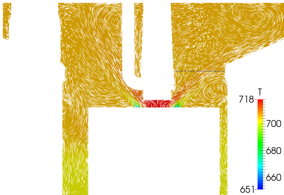
Fig. C.52: OpenFOAM: Hot pool - transient - Temperature field (0s) - velocity field
