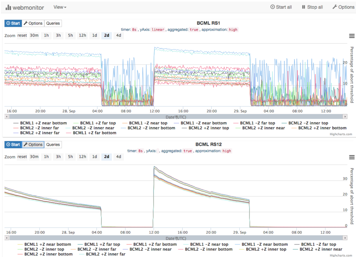
Figure A.12: The BCML web monitor displays the abort level in percent for RS1 and RS12. Two LHC fills can be seen with a duration of around 14 hours.
