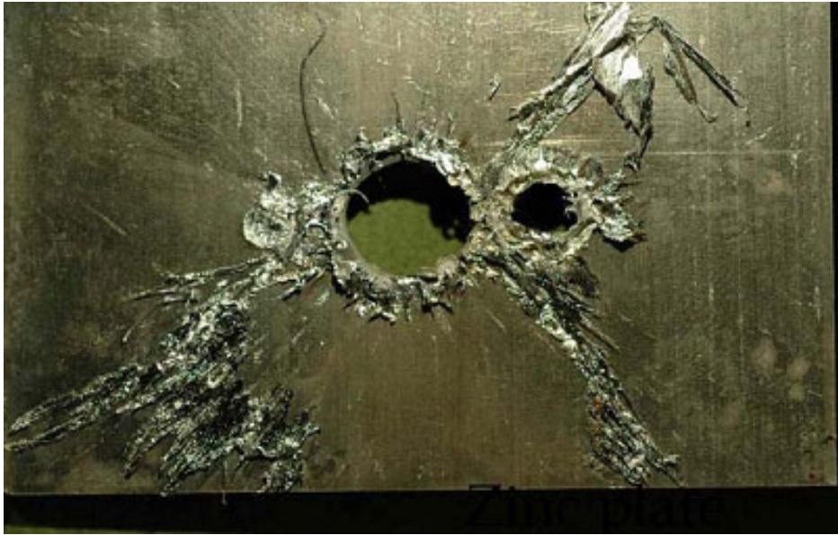
Figure 1.1: Beam loss test with 72 proton bunches at 450 GeV colliding with several 2 mm thick copper plates. The first 100 plates are destroyed by the beam loss event. Taken from [LHC16].
