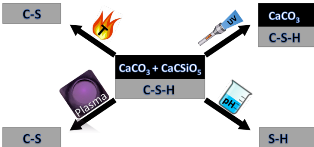
Figure 7: Schema of the results obtained by the activation of Calcium-Silicate-Hydrate phases with four different techniques: heating, UV-light exposure, plasma and wet chemical treatment.
