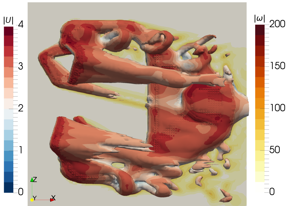
Figure 3.1.: Isosurface of the magnitude of instantaneous vorticity at time = 63 s is colored by velocity magnitude for case Y0000. The vorticity magnitude of X-Z slice is shown in the background. The wake of the transducer pin and the supporting structure are noticeable. Modified after Huq et al. (2017) (Appendix B).
