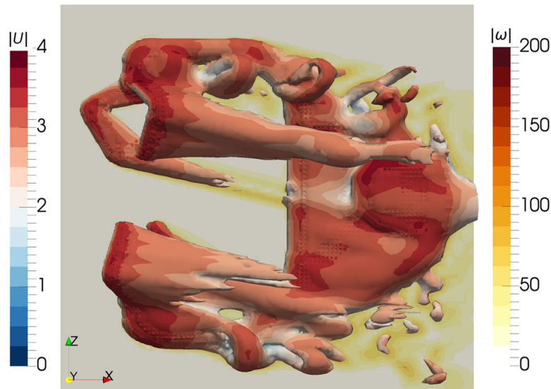
Fig. 9 Isosurface (at 66 Hz) of the magnitude of instantaneous vorticity coloured by the velocity magnitude |U| in \text{m s}^{-1} (blue to red). The background image shows the vorticity magnitude |\omega| in Hz (white to red, but only the yellow part is visible outside of the isosurface). This figure shows the case Y0000 at time = 63 s, as in Fig. 7. Only one measurement path is fully visible (upper-left transducer to lower-right transducer); the other two visible transducers are both frontal parts belonging to two different measurement paths. The corresponding transducers at the back are not visible at this viewing angle. The structure of the vortices is discussed in Sect. 4.1
