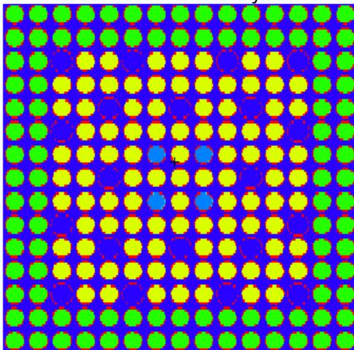
Figure 2: The Goesgen Subassembly. The 4 bright blue fuel elements in the middle depict equivalent positions of the investigated fuel segment. The water holes are seen as to some extent enlarged red cycles within the dark blue color of the simulated water. The green and yellow pins are the rest fuel pins of the subassembly.
