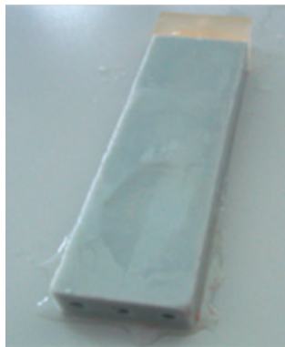
Figure 2: The agar phantom used for testing the system.
