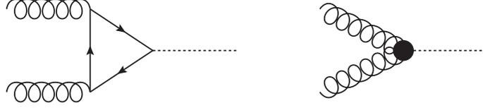
**Figure 3.2:** Diagrams for gluon fusion production of a Higgs boson. On the left the one-loop diagram with a top-quark loop is shown. Using EFT this amplitude can be expanded in the ratio  $m_h/m_t$ , which results in an effective ggh vertex.
