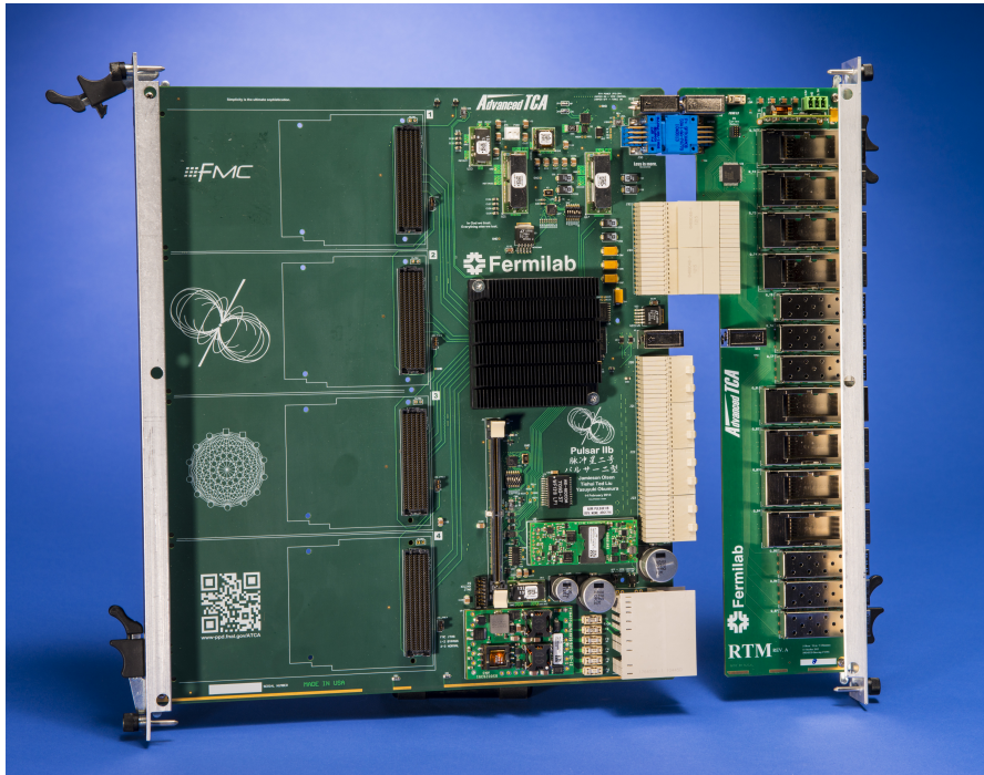
Figure 5.11.: The Pulsar IIB ATCA carrier blade with an old version of the RTM attached on the right side. Courtesy of Fermilab.
