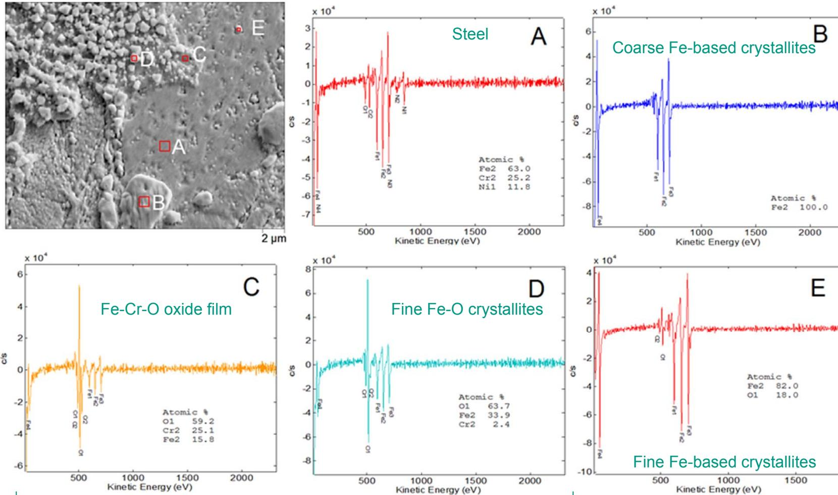
D+C = Bi-layer scale: outer magnetite + inner spinel
