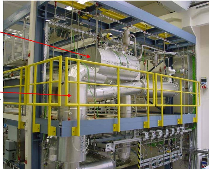
The CORRIDA facility – a forced-convection loop made of austenitic stainless steel (1.4571) designed to expose material (steel) specimens to flowing (2 m/s) Pb-Bi eutectic (~1000 kg) with controlled oxygen concentration.
