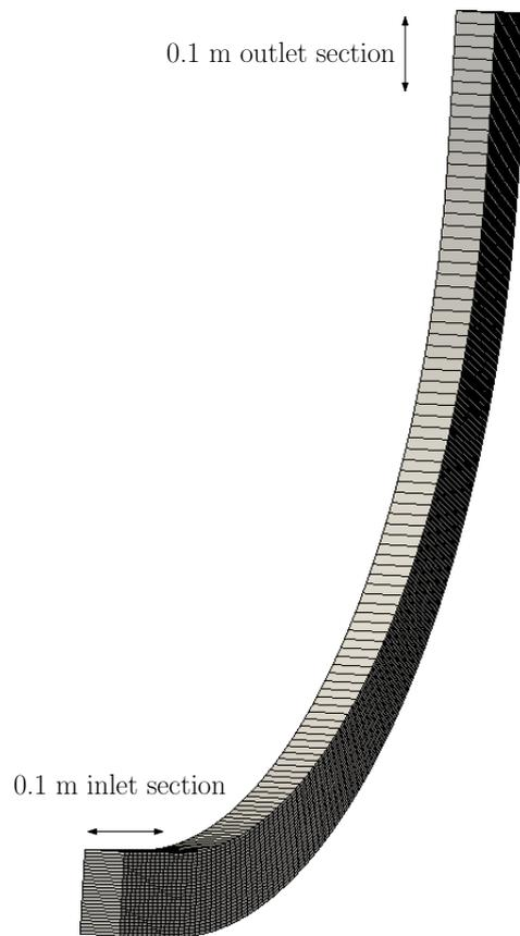
Figure 5.21: 2D mesh for the simulation of experiments by Park et al. (2013).
