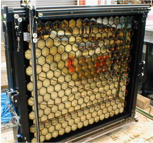
(a) The PMT camera of the TA Fluorescence Detector (TAFD)
