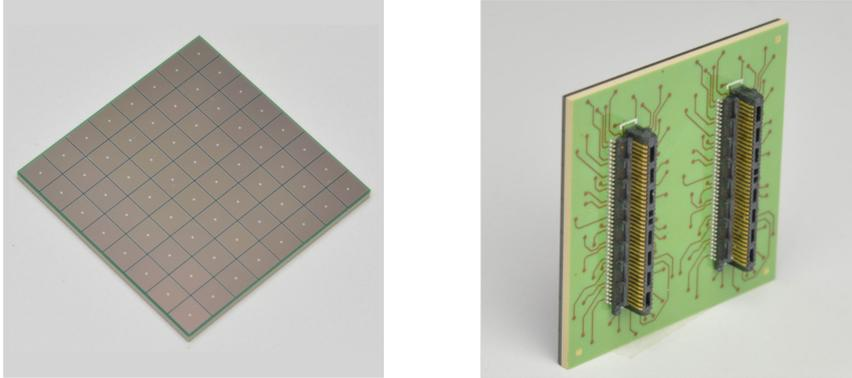
Figure 9.4: Pictures of the front and the back side of a 64-channel Hamamatsu SiPM array *S13361-3050NE*. Image taken from [92].
