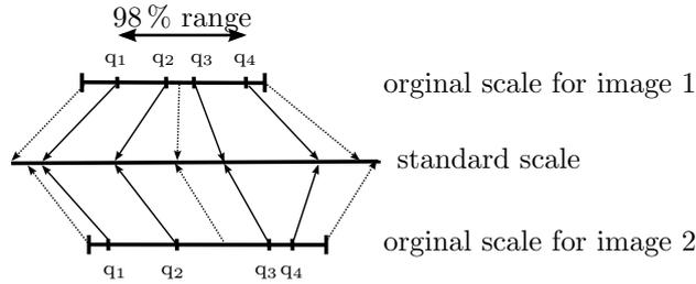
Figure 4.2: Schematic concept of the non-linear proposed by Nyúl, Udupa, and X. Zhang (2000). Within each quantile the intensity values are mapped linearly to a standard histogram, but due to the division into different quantiles, the whole process is non-linear. (Adapted from Nyúl, Udupa, and X. Zhang (2000))
