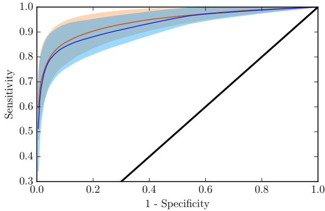
Figure 5.28: The results of the leave-one-patient-out experiments using setup I. ROC-curves for LSA<sub>2</sub> (blue) and DALSA<sub>2</sub> (red). The curves are obtained by varying the decision threshold of the classifier and then calculating the mean (solid) and standard deviation (coloured area).
