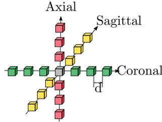
Figure 4.6: For each voxel (gray) 18 neighbours are selected, six for each direction. The neighbours are sampled with a distance  $d$ .
