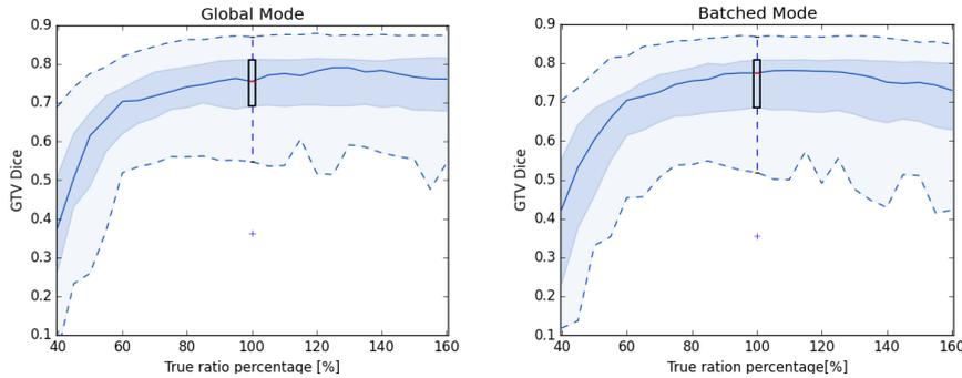
Figure 5.37: Results of leave-one-out experiments with artificially falsified  $\pi$ . All experiments are conducted with the same random forest tree depth (Global 5, Batched 4). The box in the diagram follows standard boxplot definitions and gives the results that are obtained with the true ratio.
