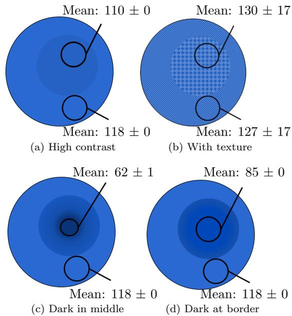
Figure 4.14: Human vision incorporates more information than only contrast. For example, it is easier to separate the two circles in (b) than in (a) although the pure contrast is higher in the latter one. Also, the ROI-placement influences the result as shown in (c) and (d)
