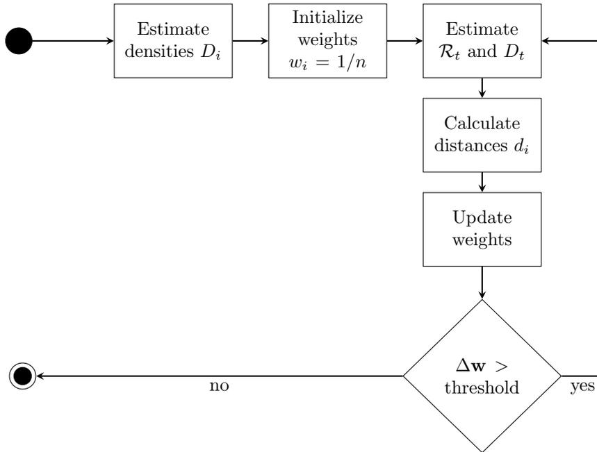
Figure 4.13: Simple work-flow for the proposed algorithm for fusing multiple ROIs. The weights are updated until the sum of differences caused in the current run are lower than a pre-defined threshold.
