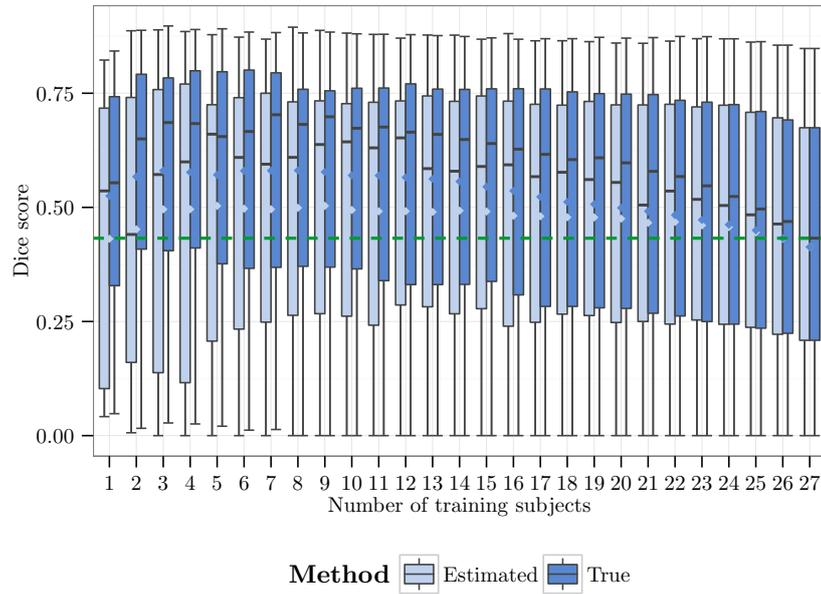
Figure 5.19: Boxplot of the obtained Dice score if the given number of best training samples are given. The results are given if the estimated, or the true, most similar training images are used. The green dashed line indicates the median result if all images are used. The notches indicate the mean value of the corresponding colour.
