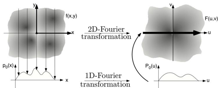
Figure 2.6: Correlation between the Radon transformation, i.e. the projection of a 2D-volume to 1D ( $p_o(x)$ ), and the 2D Fourier transformation  $F(u, v)$ . Edited reprint from Dössel (2000) with kind permission from Springer International Publishing AG.
