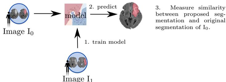
Figure 4.5: Visualization of the defined subject or image similarity. To assess the similarity of  $I_0$  to  $I_1$  a classifier is trained using  $I_1$ . Using this classifier, a segmentation is predicted for  $I_0$ . The similarity is then the overlap of the true segmentation and the predicted segmentation, measured using the Dice score.
