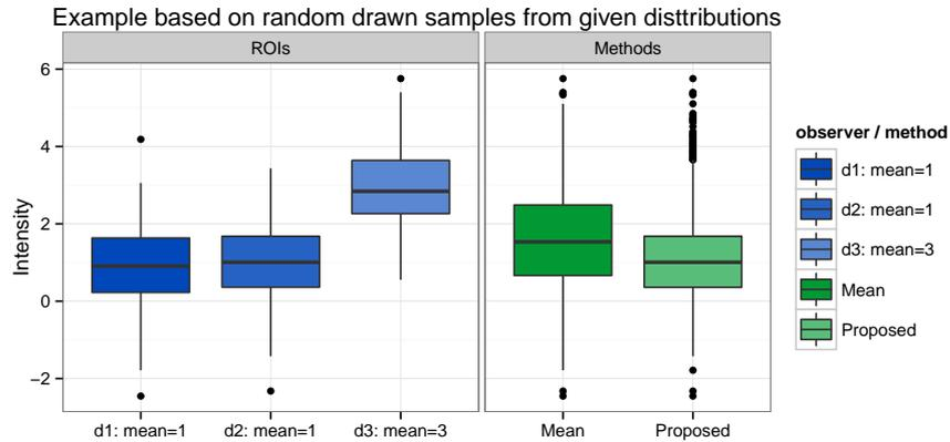
Figure 5.48: Toy example illustrating the effect of different fusion methods. Three artificial ROIs are created by randomly sampling from different normal distributions. For each ROI 200 samples are drawn with a standard deviation of 1. The results of the standard (mean) and proposed fusion are shown.
