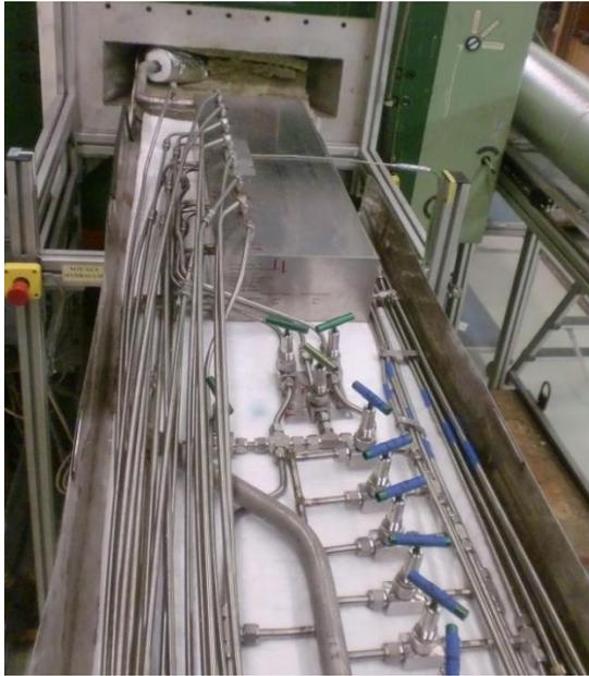
Fig. 7: Test section of a breeder unit being installed in the MEKKA facility.
