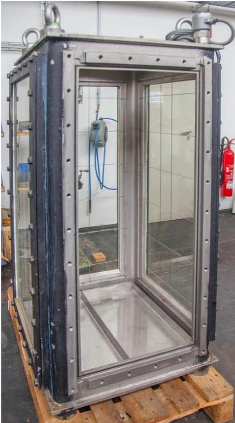
Fig. 7: DISCO vessel for visualization of the melt jet interaction with water
