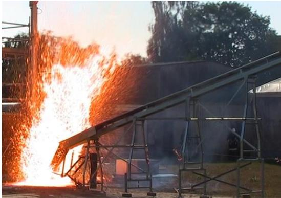
Fig. 5: Ejection of melt during the cooling process
