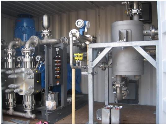
Fig. 3: Pump and heat exchanger of the organic Rankine cycle MONIKA at IKET.
