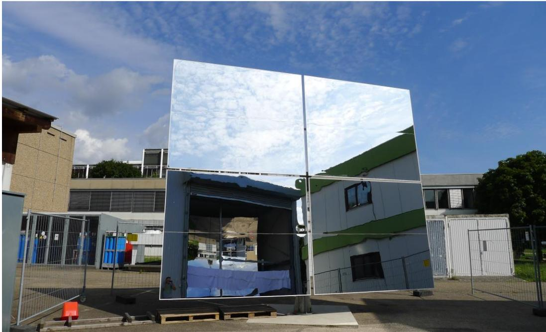
Fig. 1: Heliostat mirror of the SOMMER project, reflected in the lower left facet: the concentrating parabolic mirror.
