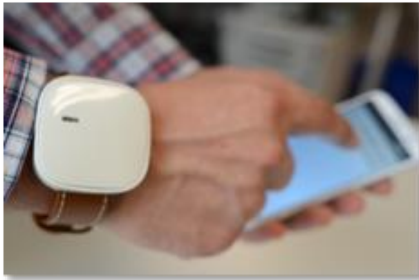
Figure 8 Wrist-worn sensor node used in the study together with the phone for data acquisition
