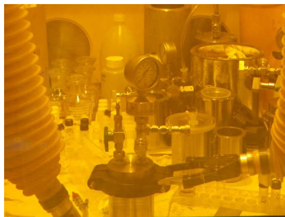
Fig. 6: Autoclave for dissolution experiments, loaded with a steel specimen, inside a shielded box. The gas-collecting cylinder is not yet connected to the autoclave.
