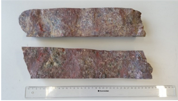
Fig. 1: Cataclased hydrothermally altered porphyroid granite of exploration well EPS-1 (K080 – bottom depth 1462.16 m).
