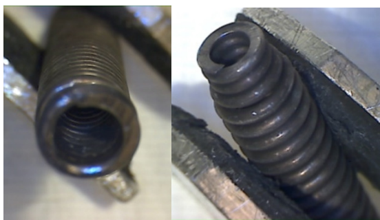
Fig. 5: Images of the irradiated stainless steel plenum spring.
