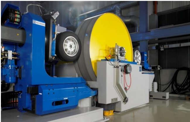
Figure 4.4: Used outer drum test bench for rolling resistance measurements
