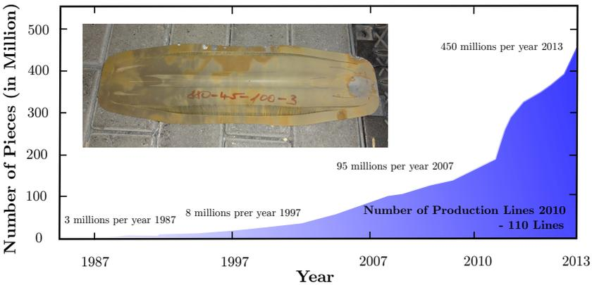
**Figure 1.1:** Development of the amount of hot stamped parts per year in automotive (Billur and Altan, 2015)
