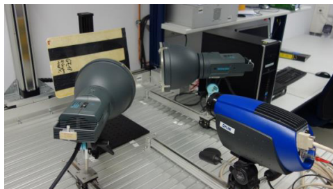
Figure 8. Test setup of thermography experiments
