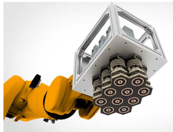
Fig. 2. Drape gripper with ten hexagonal pixels
