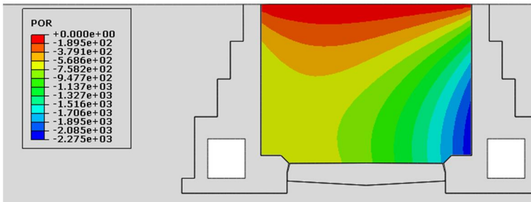
Fig. I-4 Snapshot of the hydrodynamic pressures at the time of the maximum total hydrodynamic pressure.
