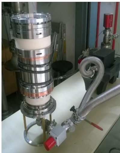
Fig. 2. Assembled Inverse Magnetron Injection Gun during the bake out process
