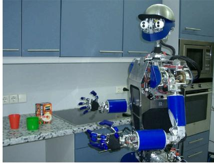
**Figure 1.5.** *The humanoid robot ARMAR III developed by [Asfour et al. \(2006\)](#) serves as the main target application of the activity recognition system developed in the context of this work. Goal of the proposed approach is to enable an implicit, non-verbal communication of a human with the robot through the recognition of activities based on the analysis of image sensor data (©2006 IEEE).*
