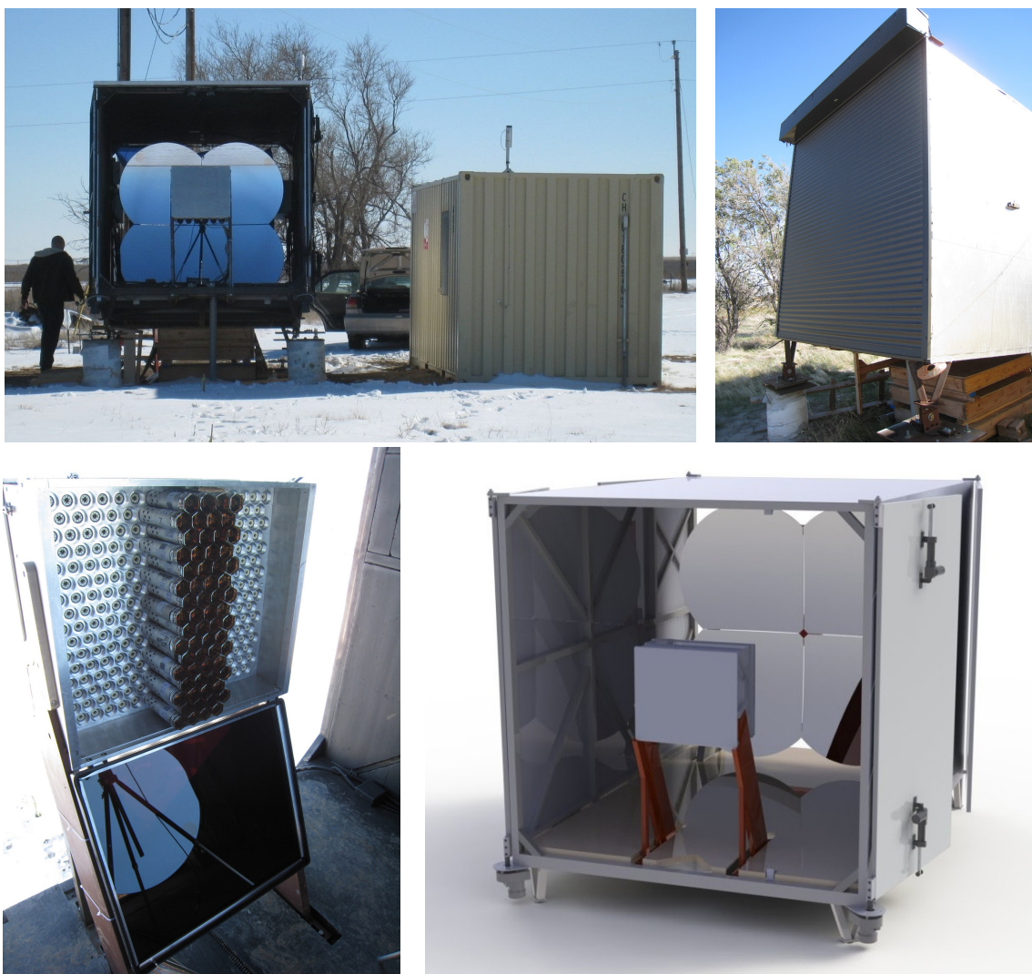
Figure 7. AMT mirror, camera, weather sensors and calibration system are housed in a custom shelter (top left), the adjacent container contains the data acquisition system. A roll-up door can be closed across the entrance aperture (top right). The AMT camera (bottom left) is shown with the UV bandpass optical filter opened. A 3D rendering of the AMT using the CAD design software SolidWorks® (bottom right).
