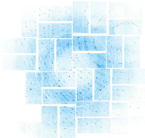
Figure 54: Diffraction image from a single nanocrystal built from the protein lysozyme [AHC14]. The distribution of the rectangles corresponds to the location of the sub-panel within the front panel at the LCLS. The dark spots show the Bragg-spots. The photon background is given by the “halo ring” around the beamhole at the centre of the detector.
