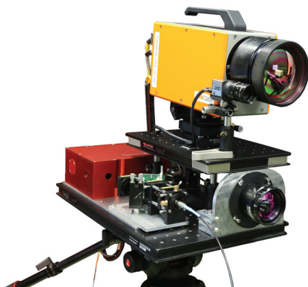
Figure 6.2: The short range hyperspectral image sensor can be operated between 20 cm and 5 m and provides a spectral tuning range of 1000 cm -1 to 1300 cm -1 .
