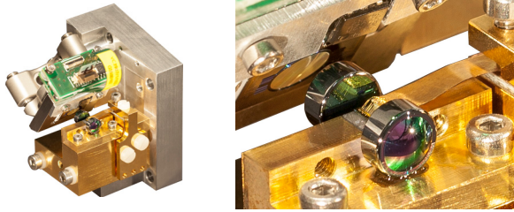
Figure 8.2: MOEMS EC-QCL light source that was developed in collaboration with Fraunhofer IPMS. Left: compact design allows integration into measurement systems with a small footprint. Right: close-up of laser chip with collimation lenses in external cavity resonator and MOEMS grating.
