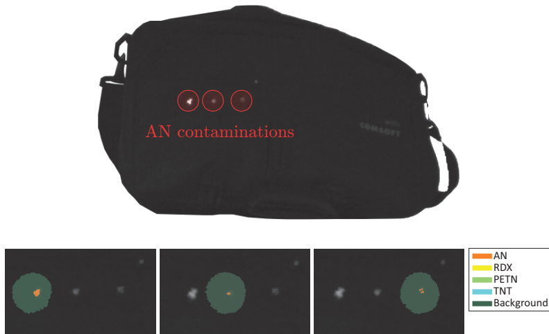
Figure 7.23: Top: Polyamide carrying bag containing several Ammonium Nitrate contaminations. Bottom: detection results obtained using the long range hyperspectral image sensor from a distance of \approx 17 m. All AN contamination areas were successfully detected by the AMSD-ABGP detection algorithm.
