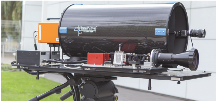
Figure 6.3: The long range hyperspectral image sensor is operational in the range of 10 m to 25 m and equipped with a CMOS camera aligned to the collection optics that provides a visible image of the scene along with the hyperspectral image.
