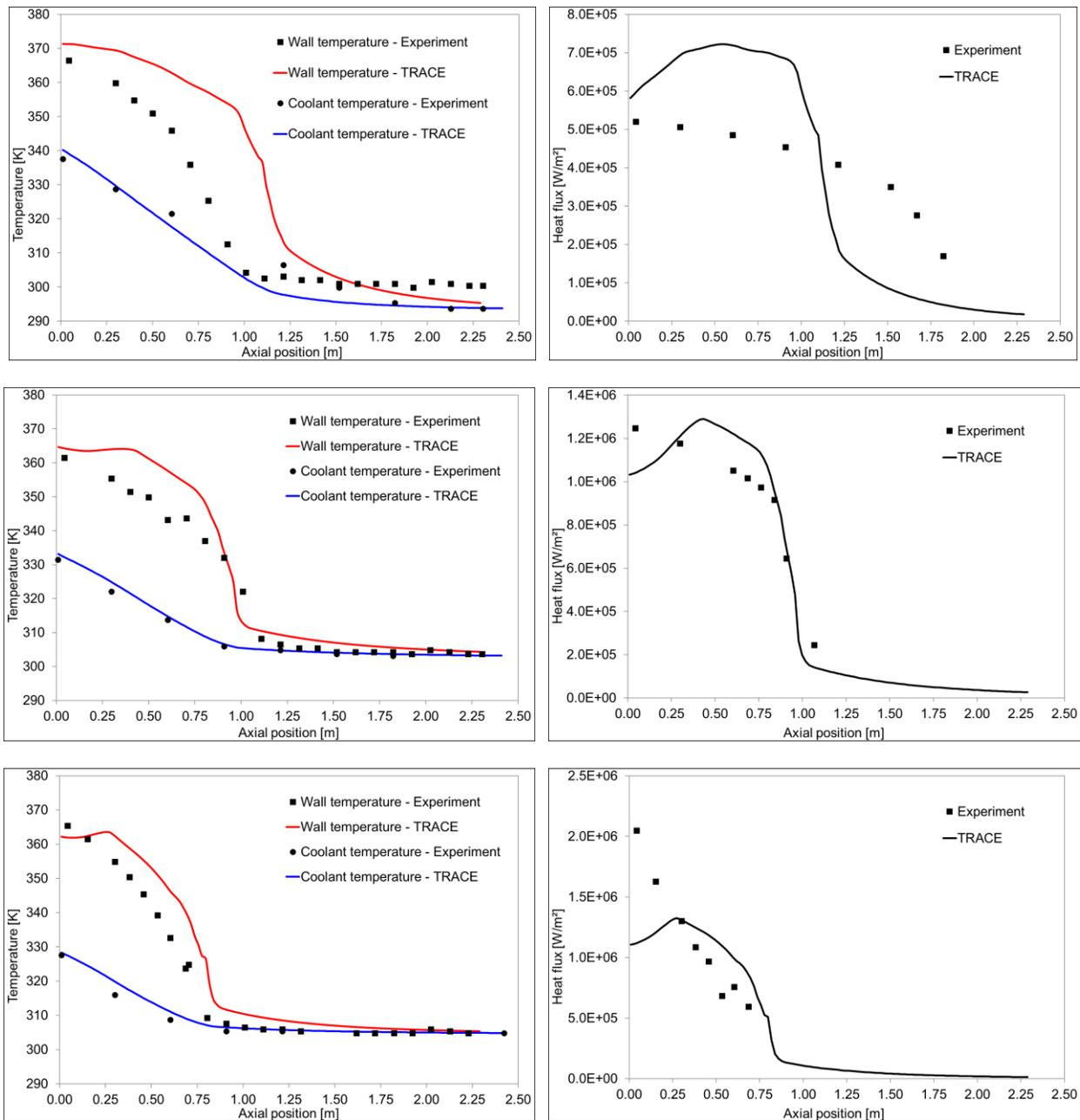
Figure 4 Experimental data (symbols) in comparison to TRACE calculations (lines) for the inner wall temperature of the inner tube, the coolant temperature (both on the left diagrams) and the heat flux from the inner tube to the outer tube (on the right diagrams as a function of the axial length for test runs 176 (top), 209 (center) and 229 (bottom))
