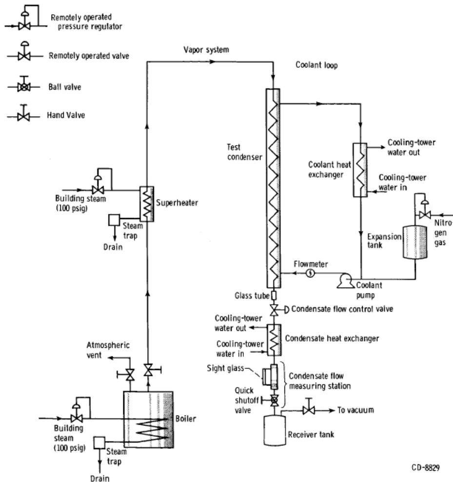
Figure 1 Schematic drawing of the test facility [5]
