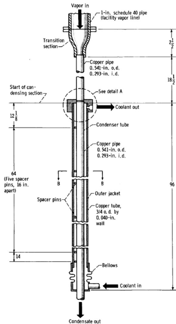
Figure 2 Tube-in-tube test section (dimensions in inch) [5]
