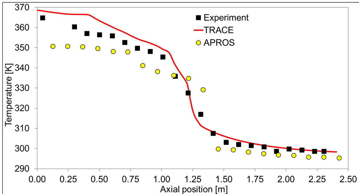
Figure 6 Wall temperature as a function of the axial length for test run 163 - Comparison of experimental results and calculations with TRACE and APROS
