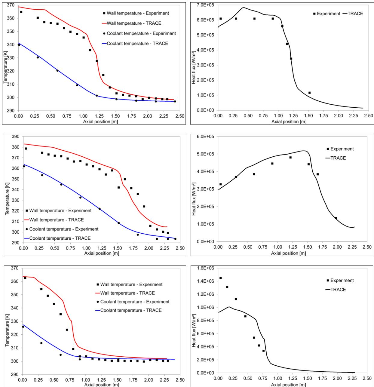
Figure 3 Experimental data (symbols) in comparison to TRACE calculations (lines) for the inner wall temperature of the inner tube, the coolant temperature (both on the left diagrams) and the heat flux from the inner tube to the outer tube (on the right diagrams) as a function of the axial length for test runs 163 (top), 167 (center) and 170 (bottom)
