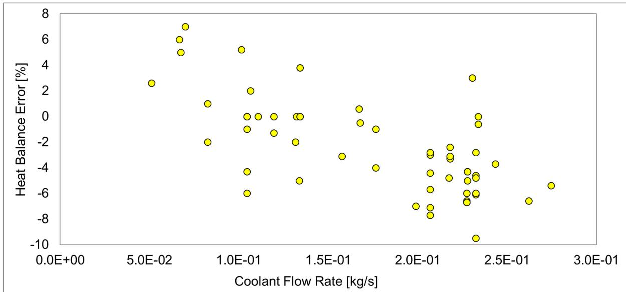
Figure 5 Heat balance error as a function of the coolant mass flow rate for all 58 test runs
