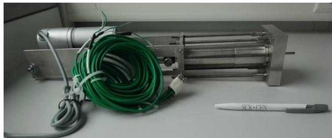
Figure 2: First prototype of the permanent magnetic probe.
