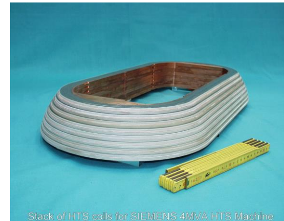
Stack of HTS coils for SIEMENS 4MVA HTS Machine
