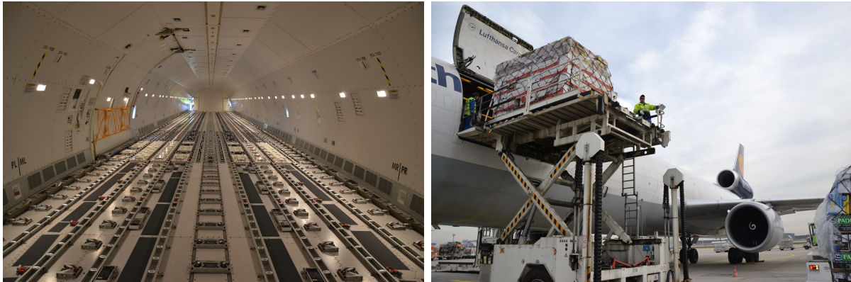
Figure 2.7: Aircraft loading: Empty main deck of a cargo aircraft with rollers and latches on the floor (left). Loading of packed ULDs into the aircraft (right). Source: Lufthansa Cargo AG, Photographer: Jannah Baldus (right)
