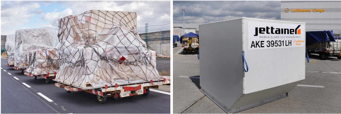
Figure 2.2: Loaded PMC pallet with main deck contour (left). Lower deck AKE container (right). Source: Lufthansa Cargo AG, Photographer: Stefan Wildhirt (left), Ingrid Friedl (right)
