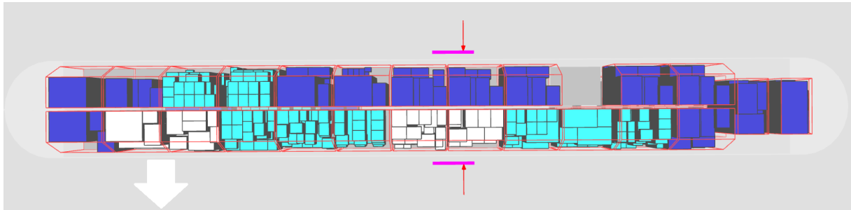
(a) After leg 1/3: Four ULDs (white) need to be unloaded. Therefore, three additional ULDs must be temporarily removed.
