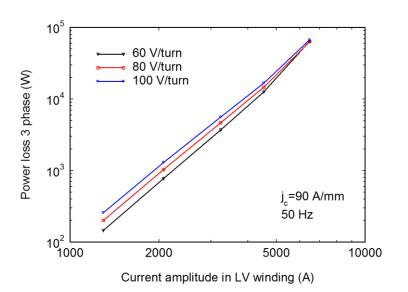
Calculated AC loss for 40 MVA design; loss increases as  $I^{3.5}$
