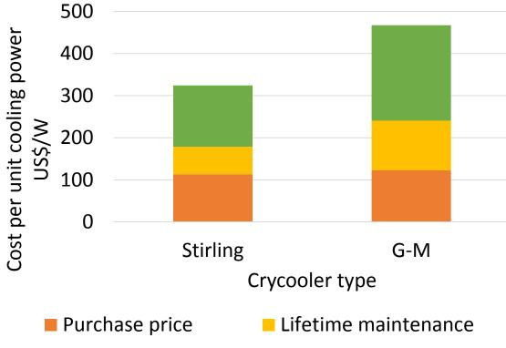
The figure of merit is the TCO per watt of cooling power, calculated here for:
