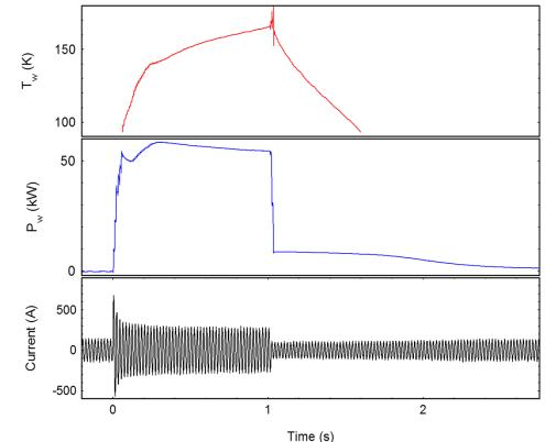
45 kVA FCL transformer winding, 0.4 mm thick wire: Heat transferred by boiling ≈ heat capacity
