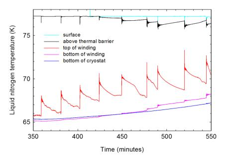
45 kVA FCL transformer winding: 2 K temperature rise of nitrogen at winding top at each short circuit, but surface liquid hardly affected
