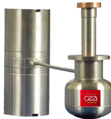
LPT9310 COTS cooler Pulse tube 5 W @ 77K <7.0 kg
