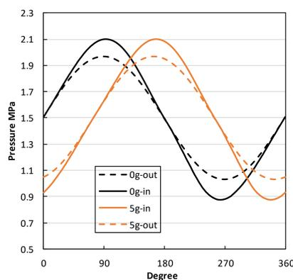
Fig.17 Pressure waves at the inlet and outlet of regenerator
