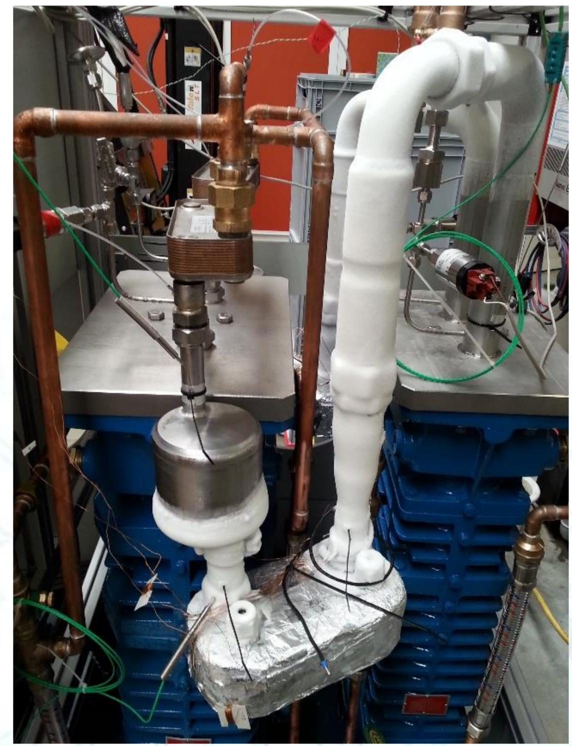
High capacity pulse tube cryo cooler at test stand
