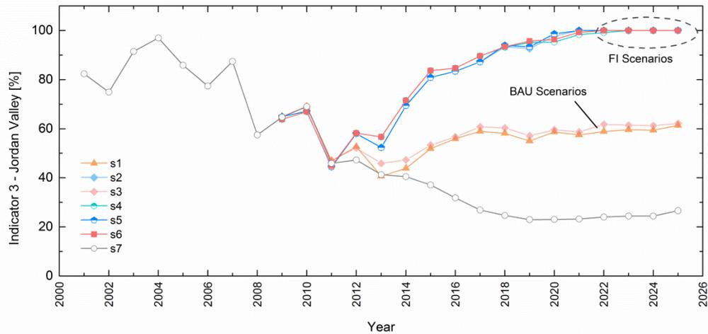
Fig. 4.12 Covered supply for external demand site representing groundwater flows that leave the model domain in the Jordan Valley through the western and southern boundaries.
