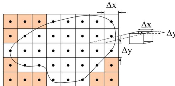
Fig. 1.5 Two-dimensional horizontal finite difference grid centred in the cell, where the contour represents the model domain, *white* cells are active and *orange* cells inactive. Based on Anderson et al. (2015).
