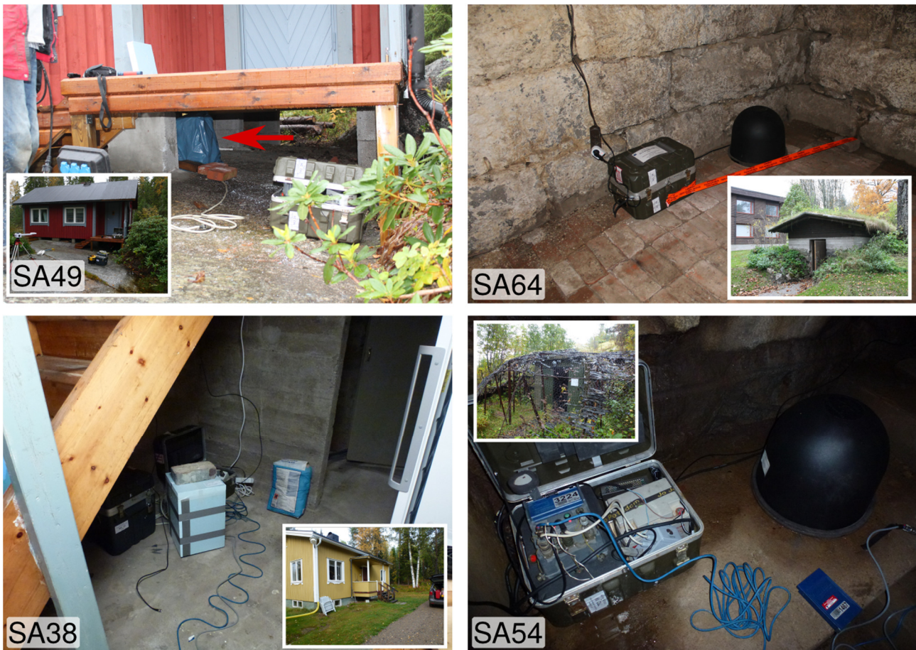
Figure 2: Exemplary instrument installations at recording stations SA49, SA64, SA38 and SA54. At station SA49 the sensor (red arrow) was installed underneath the building. At stations SA64, SA38 and SA54 cellars were used. The sensors were protected with insulation material against temperature variations.
